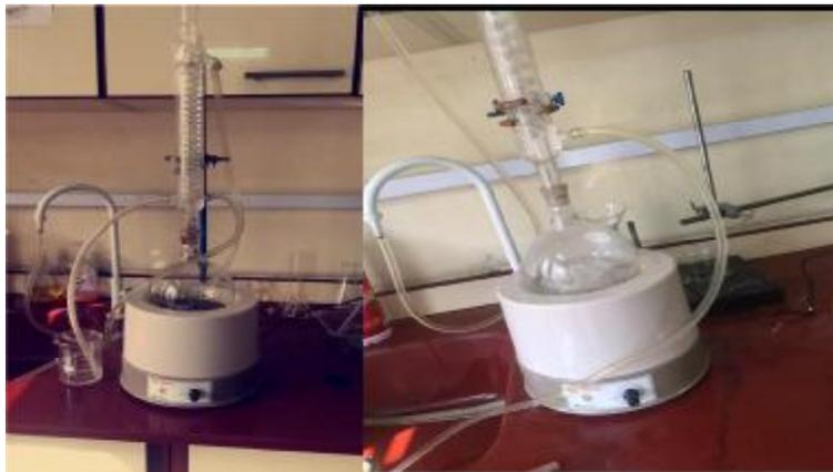
Figure (1): Reflux apparatus (Close system).
