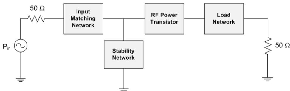
**Figure (11): Block Diagram of the RF Power Amplifier.**
