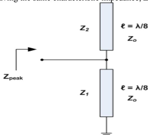
**Figure (4): Impedance Peaking Circuit.**
