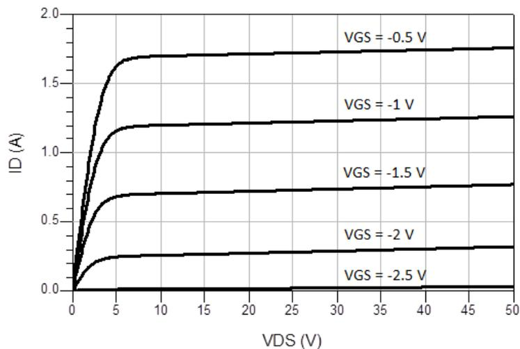
Figure (9): Drain Current versus Drain-to-Source Voltage.
