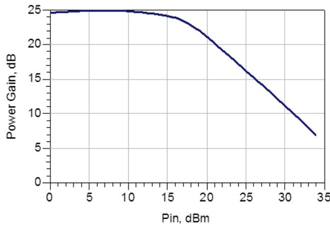
Figure (19): Simulated Power Gain versus Input Power.
