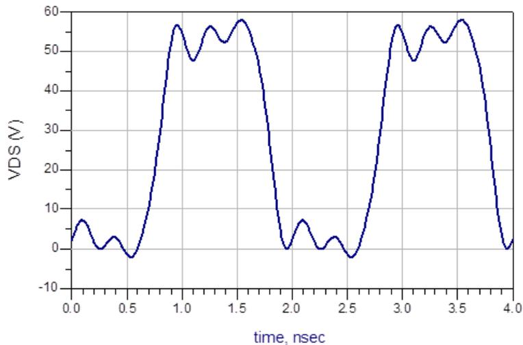
Figure (15): Simulated Drain Voltage Waveform at 500 MHz.
