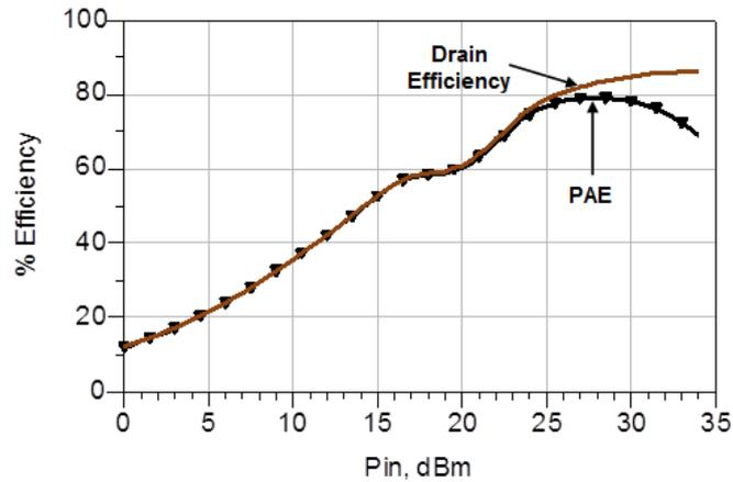
Figure (20): Efficiency versus Input Power.
