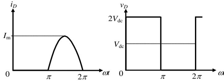
**Figure (1): Idealized Waveforms of the Drain Current and Voltage in the Class F Power Amplifier.**
