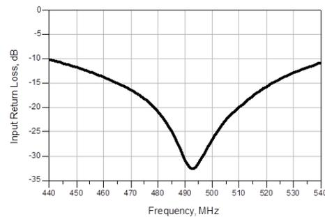
Figure (24): Input Return Loss versus Frequency.
