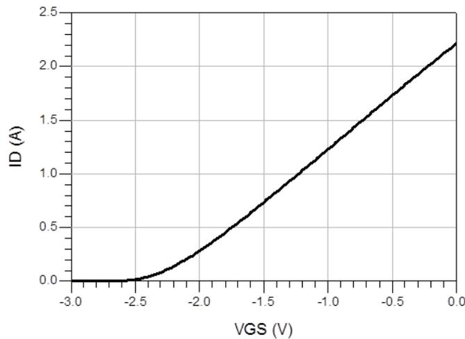
Figure (8): Drain Current versus Gate Voltage for the GaN HEMT Transistor.
