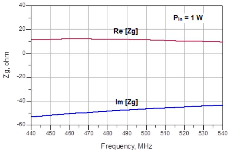
Figure (13): Simulated Gate Impedance versus Frequency.
