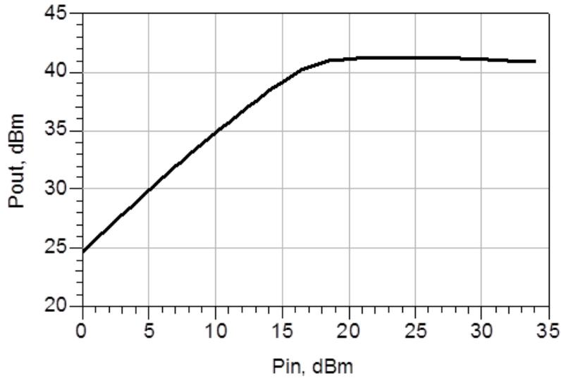
Figure (18): Output Power versus Input Power.
