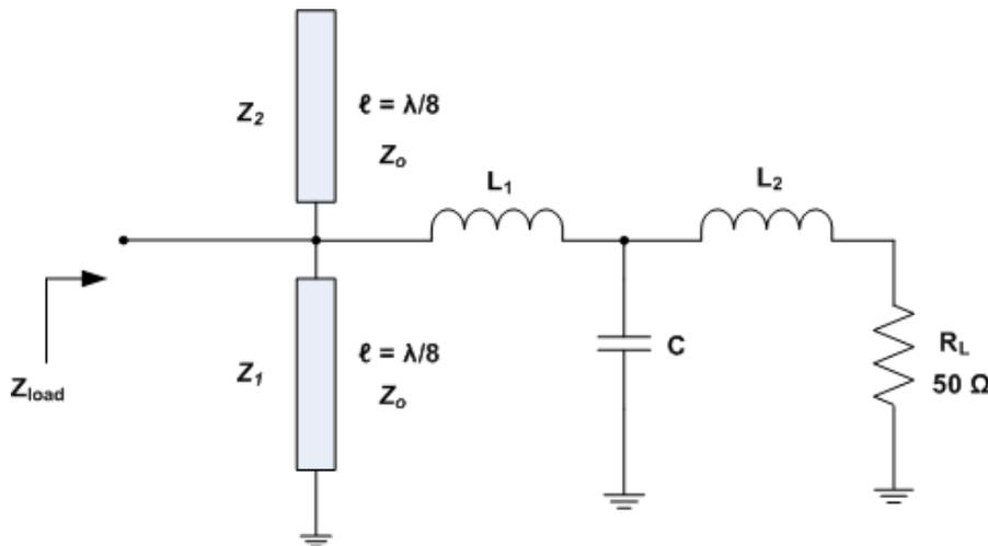
Figure (7): Configuration of the Proposed Load Network.
