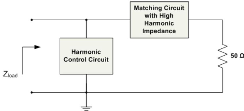
**Figure (3): General Topology of the Load Network.**
