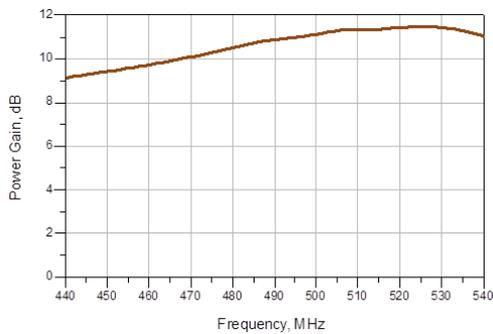
Figure (21): Power Gain versus Frequency.
