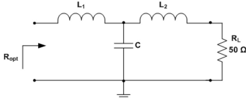
Figure (6): T-Section Matching Network.
