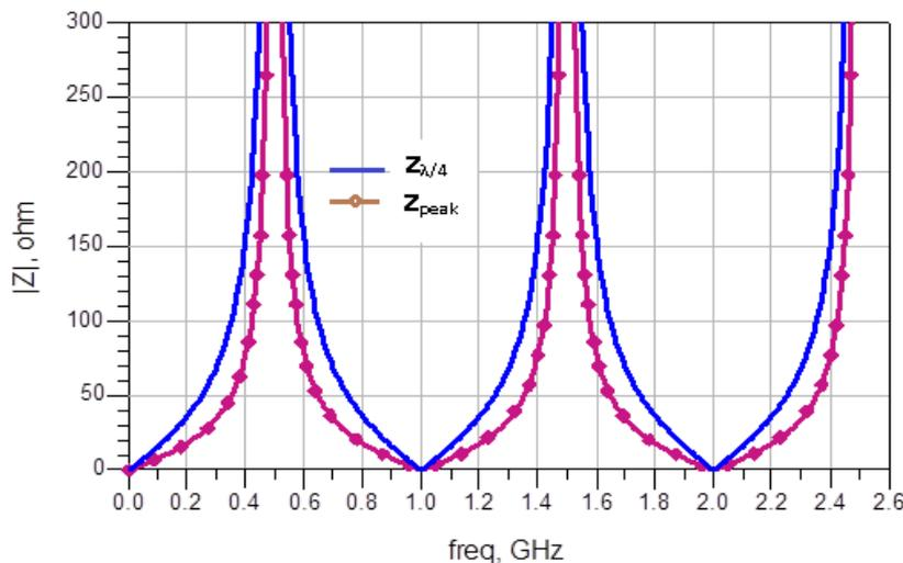
**Figure (5): Impedance Response of the Suggested Harmonic Peaking Circuit Compared with that of the Shorted  $\lambda/4$  Transmission Line.**
