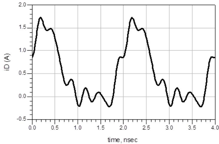
**Figure (16): Simulated Drain Current Waveform at 500 MHz.**
