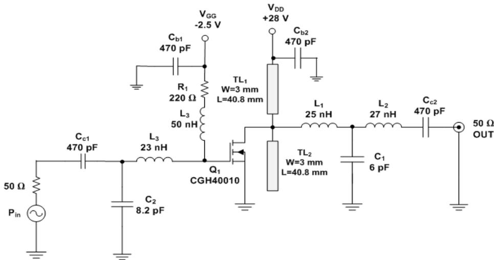
Figure (14): Schematic Diagram of the Designed Class F Power Amplifier.
