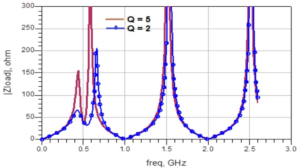
**Figure (10): Impedance Response of the Load Network with Different Quality Factors.**
