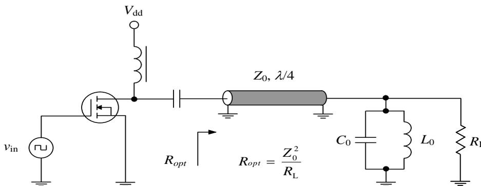
**Figure (2): Schematic Diagram of the Conventional Class F RF Power Amplifier.**
