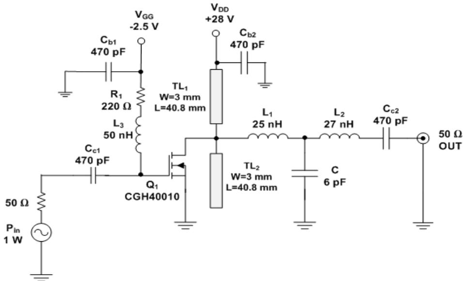
Figure (12): Circuit Schematic of the Class F Power Amplifier without the Input Matching Network.
