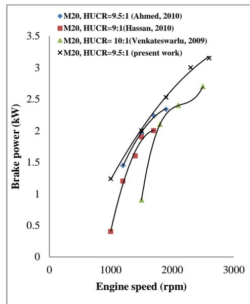
**Fig. 20, Engine speed effect on BP for comparison with other researches at HUCR and OST for M20 fuel and constant speed**
