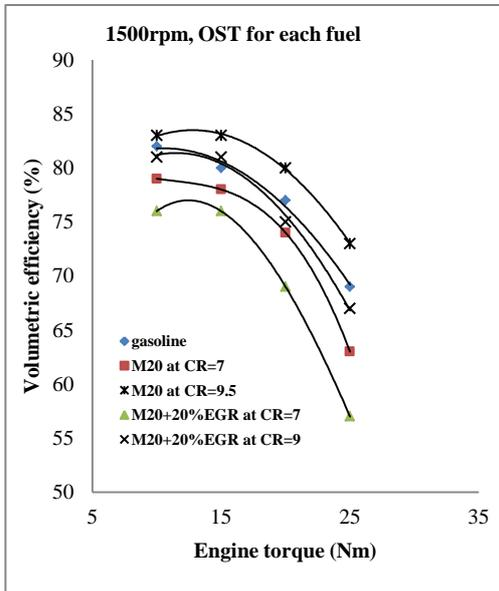
**Fig. 17, Engine torque effect on volumetric efficiency for studied cases at HUCR and OST for each fuel and constant speed**
