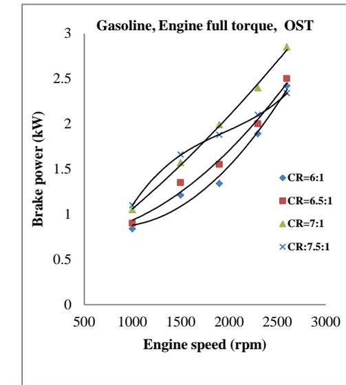
Fig. 4, Compression ratio effect on BP for gasoline at variable speed and OST and constant torque
