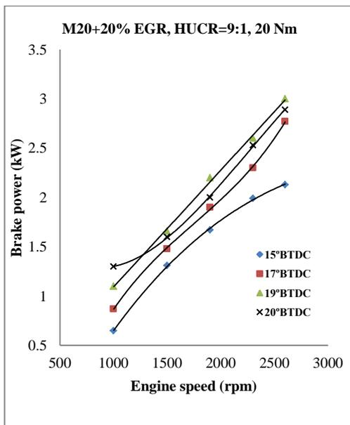
**Fig. 9, Spark timing effect on BP for M20+20% EGR at variable speed**
