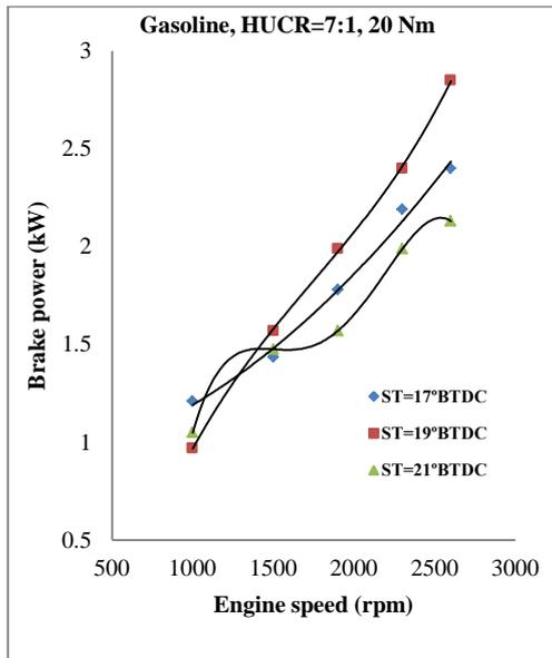
**Fig. 7, Spark timing effect on BP for gasoline at variable speed, HUCR and constant torque**
