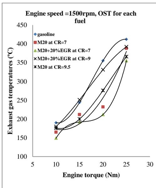
**Fig. 19, Engine torque effect on exhaust gas temperatures for studied cases at HUCR and OST for each fuel and constant speed**
