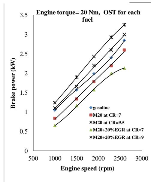
**Fig. 10, Engine speed effect on BP for studied cases at HUCR and OST for**
