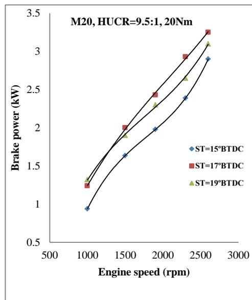
**Fig. 8, Spark timing effect on BP for M20 blend at variable speed, HUCR and constant torque**
