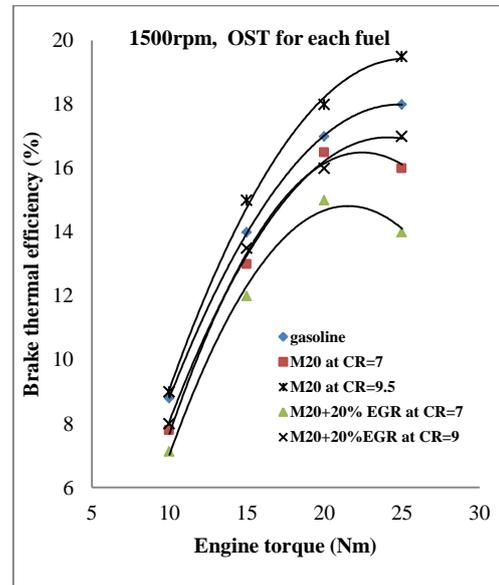
**Fig. 18, Engine torque effect on brake thermal efficiency for studied cases at HUCR and OST for each fuel and constant speed**
