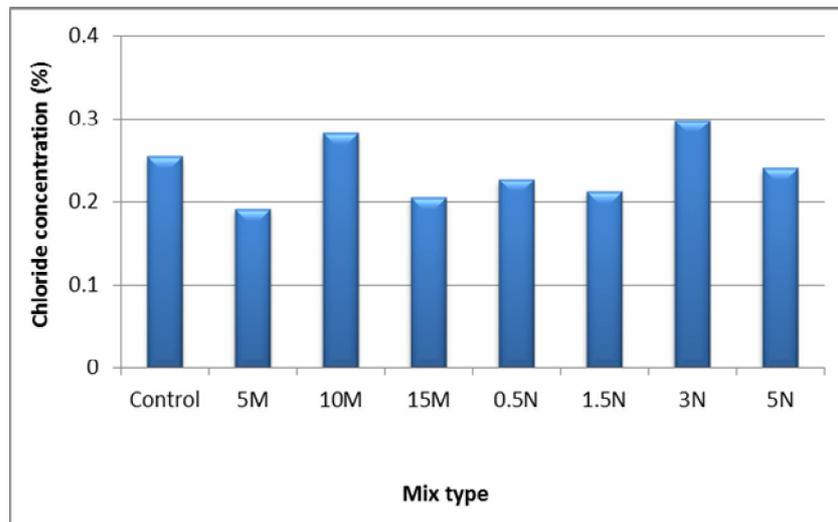
Figure 3: chloride content of concrete mixes after 23 weeks of wetting-drying exposure.
