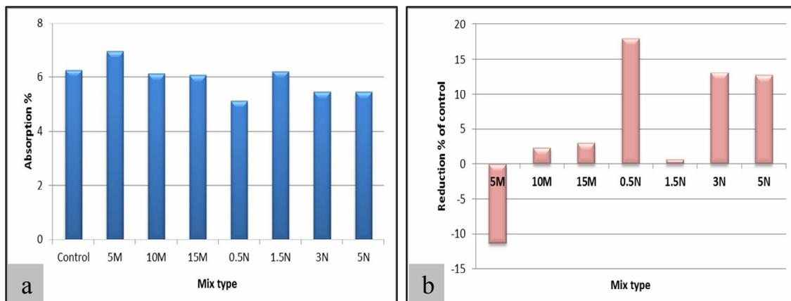
Figure 5: (a) Water absorption %; and (b) Reduction % of control mixes
