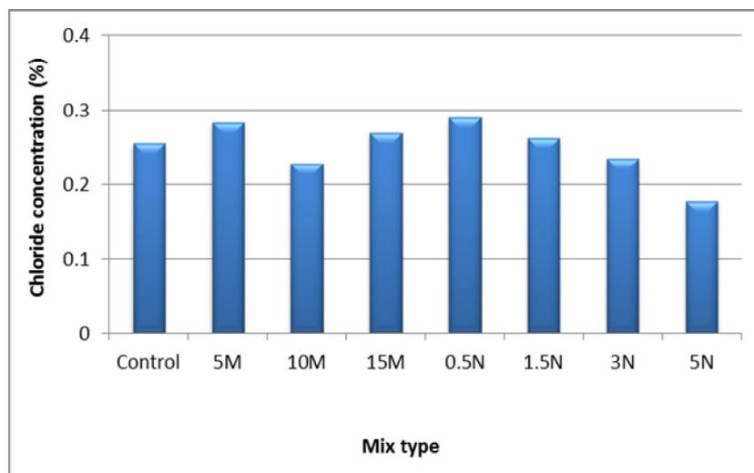
Figure 4: chloride content of concrete mixes after 23 weeks of full immersing exposure.
