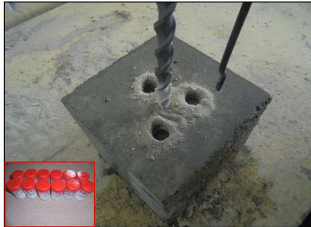
Figure 2: Concrete drilled holes for chloride content test.
