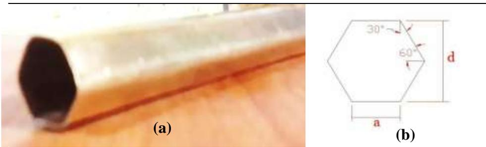
Fig. 2. (a) Hexagonal duct used in the present study. (b) Sketch of hexagonal cross section.
