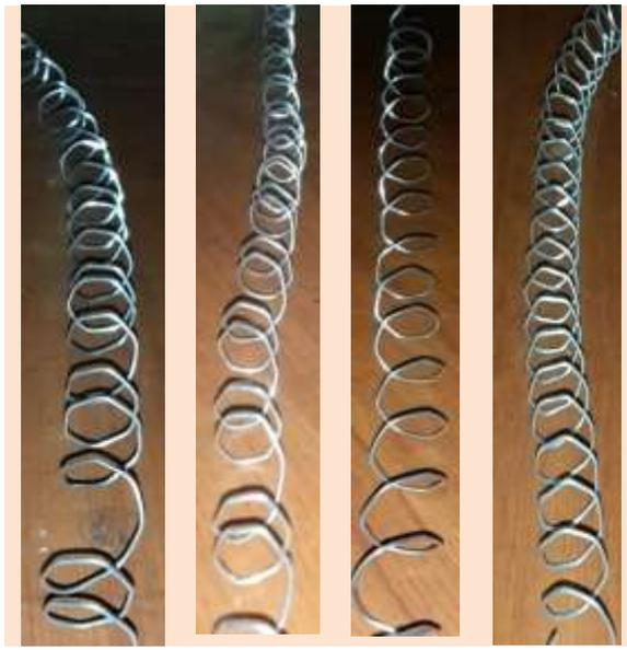
I D-coil      I-coil      P=20mm      P=10mm
