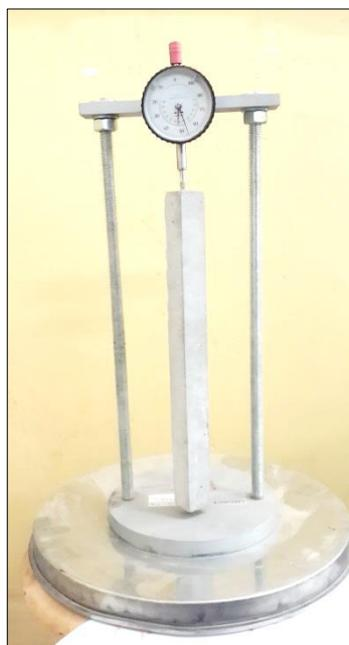
Plate (4): Drying shrinkage apparatus.
