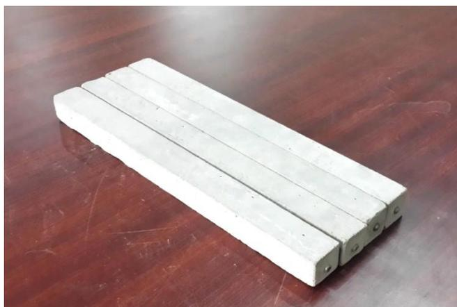
Plate (3): Drying shrinkage specimens.
