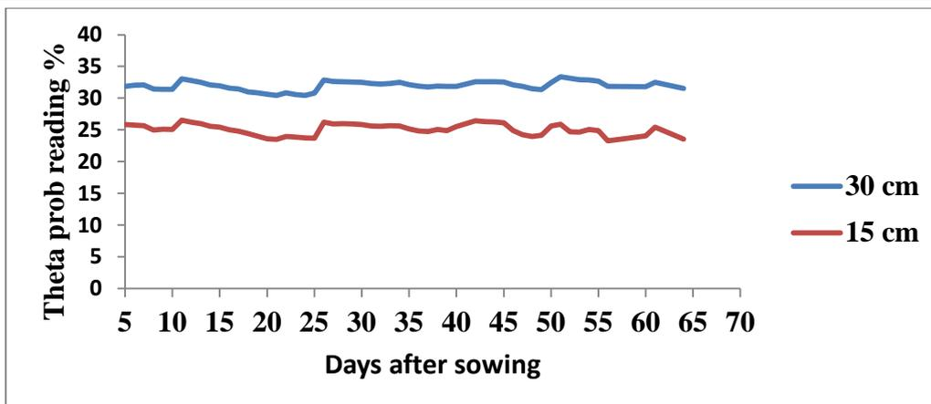
Figure 3: The average theta probe reading against the days after sowing with two different depths 15 cm with red line and 30 cm with blue line.
