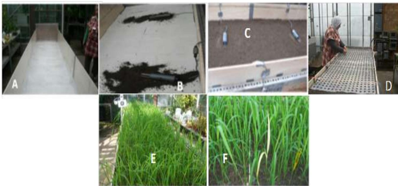
Figure 1: A; Above the saturated soil, a layer of filter papers was laid which had been soaked in 56g of TRIK in 300 ml of water and then dried; B; Above the filter paper was placed two theta probes; C; At depth 15 cm two theta probe was placed; D; The box was filled with top soil leaving 5 cm at the top and a plastic sheet containing perforations (2 cm diameter) for sowing plants at a 5 x 5 cm spacing was placed on top; E
