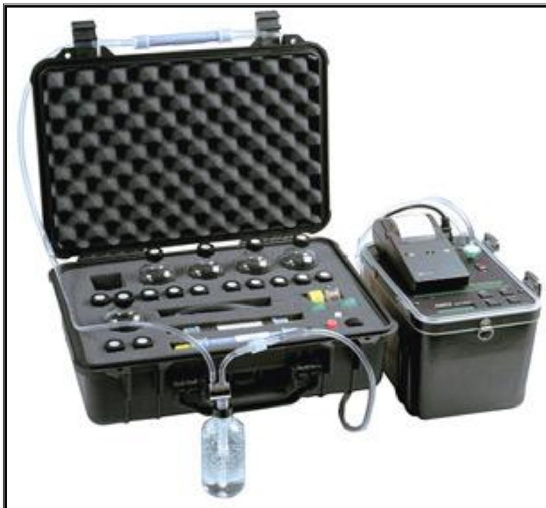
Fig. (2): Photo showing arrangement of of apparatus for measuring radon content in water sample in a 250 mL via [7]
