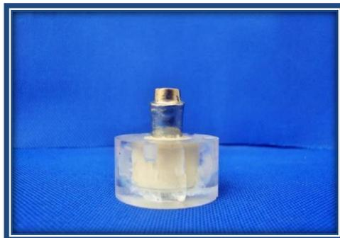
**Figure 2: Master Metal die fixed to acrylic base**
