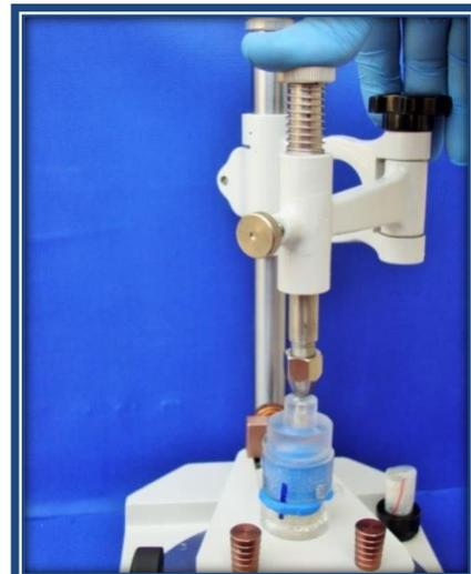
**Figure 3: Impression making with dental surveyor.**
