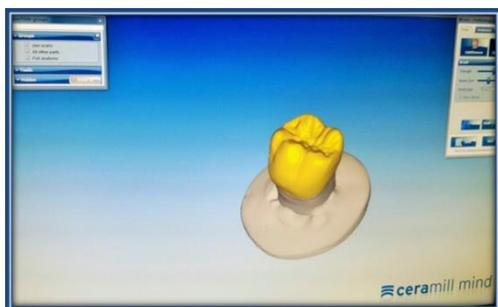
Figure 4: Final crown design before milling
