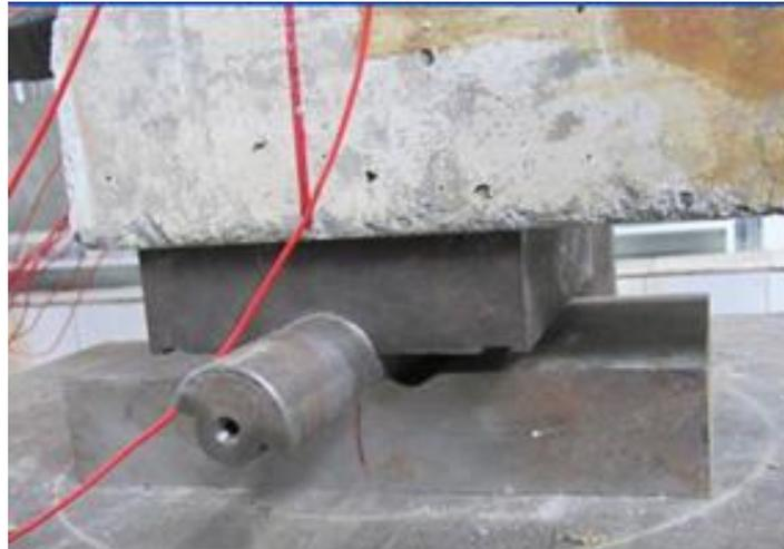
Figure 4. Specimen support with roll-plate.
