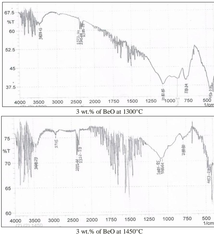
Figure 4- FTIR spectra of porcelain samples containing 3 and 7 wt% BeO at different sintering temperature.
