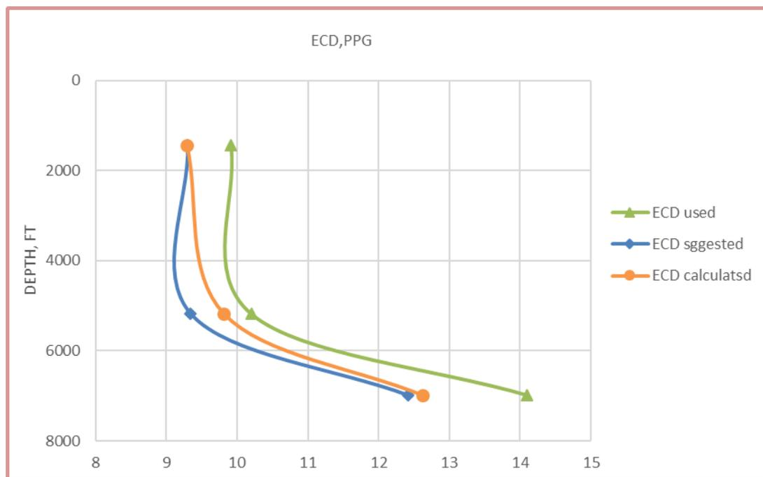
**Figure 4-** Comparison between used ECD, calculated ECD and suggested ECD
