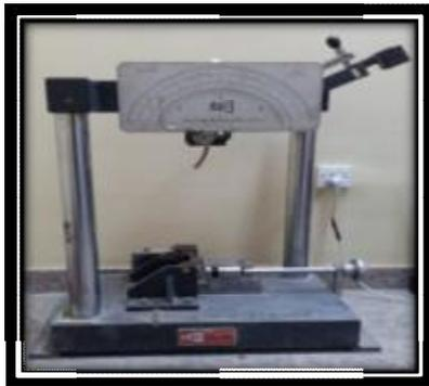
Figure 3: Impact testing devise (charpy type)
