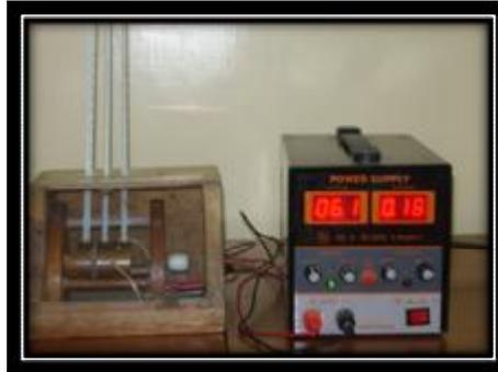
Figure 7: Thermal conductivity testing apparatus.
