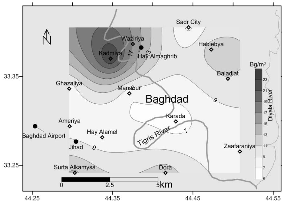
**Figure 6-** contour map shows the distribution of radon in city of Baghdad. Contour interval is 2 Bq/m<sup>3</sup>.
