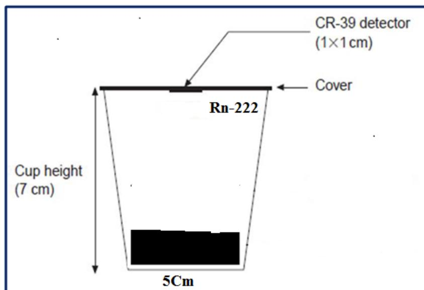
Figure 1- Radon gas ( $^{222}\text{Rn}$ ) estimation by using (CR-39) detector.
