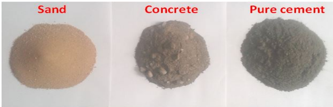
Fig. (3) Samples of storage heat materials used in this work
