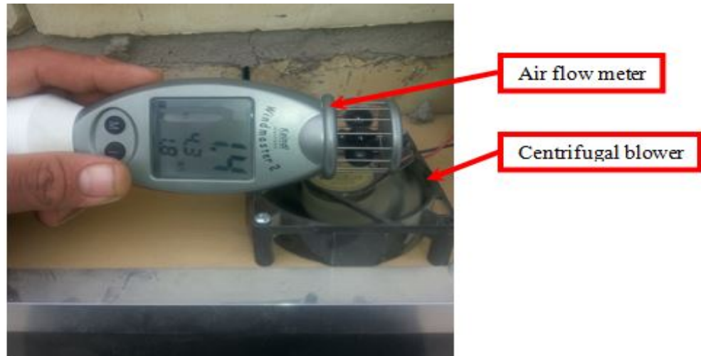
Fig. (2) Air velocity meter with centrifugal blower
