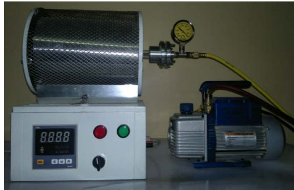
Fig.2 : The tubular furnace of 1200 °C maximum temperature used in this study
