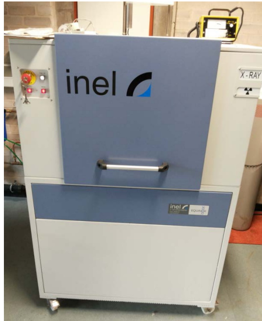
Fig.5 : Inel Equinox 3000 X-Ray Diffractometer used in this study.
