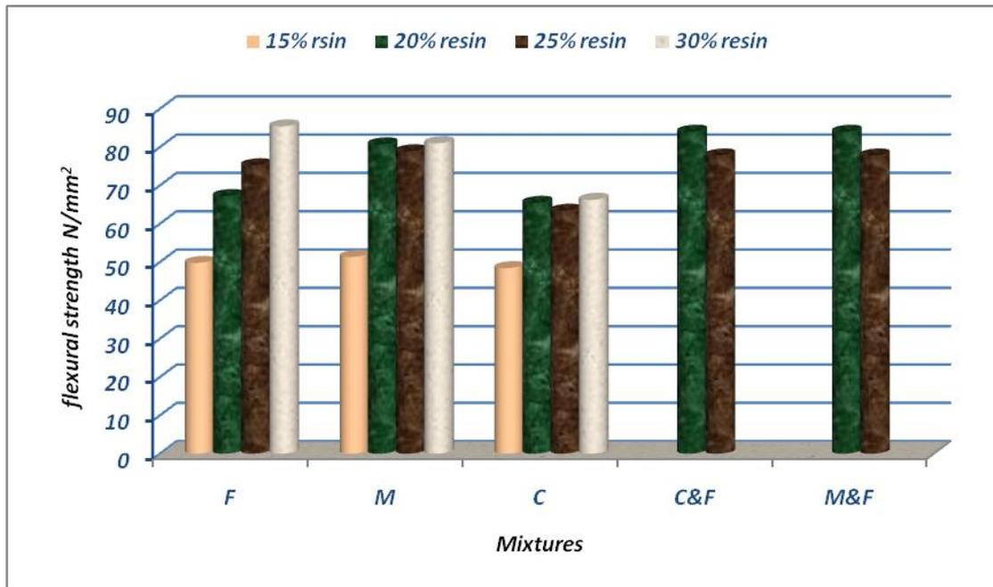
**Figure 3-** flexural strength results of polymer concert.
