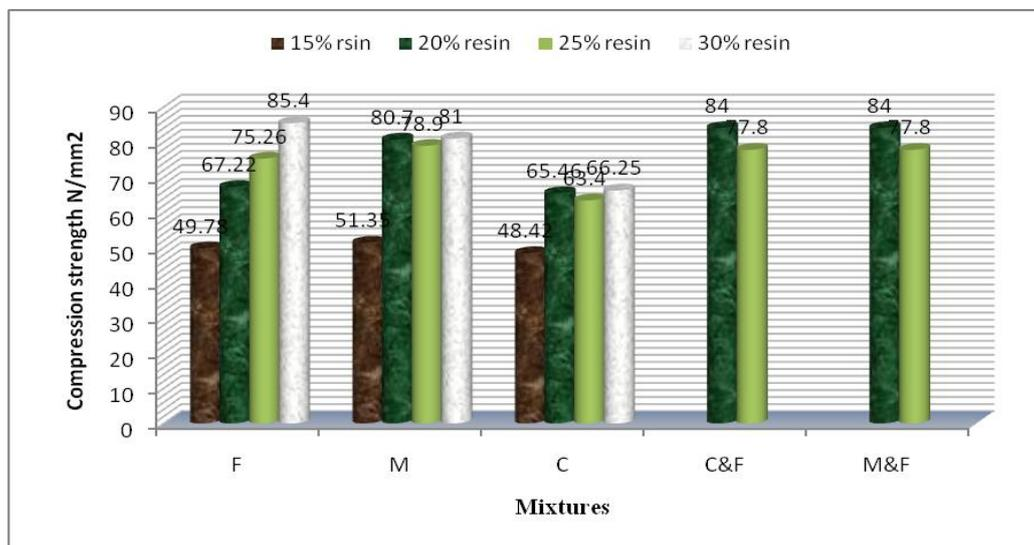
**Figure -1** compression strength results of polymer concrete .
