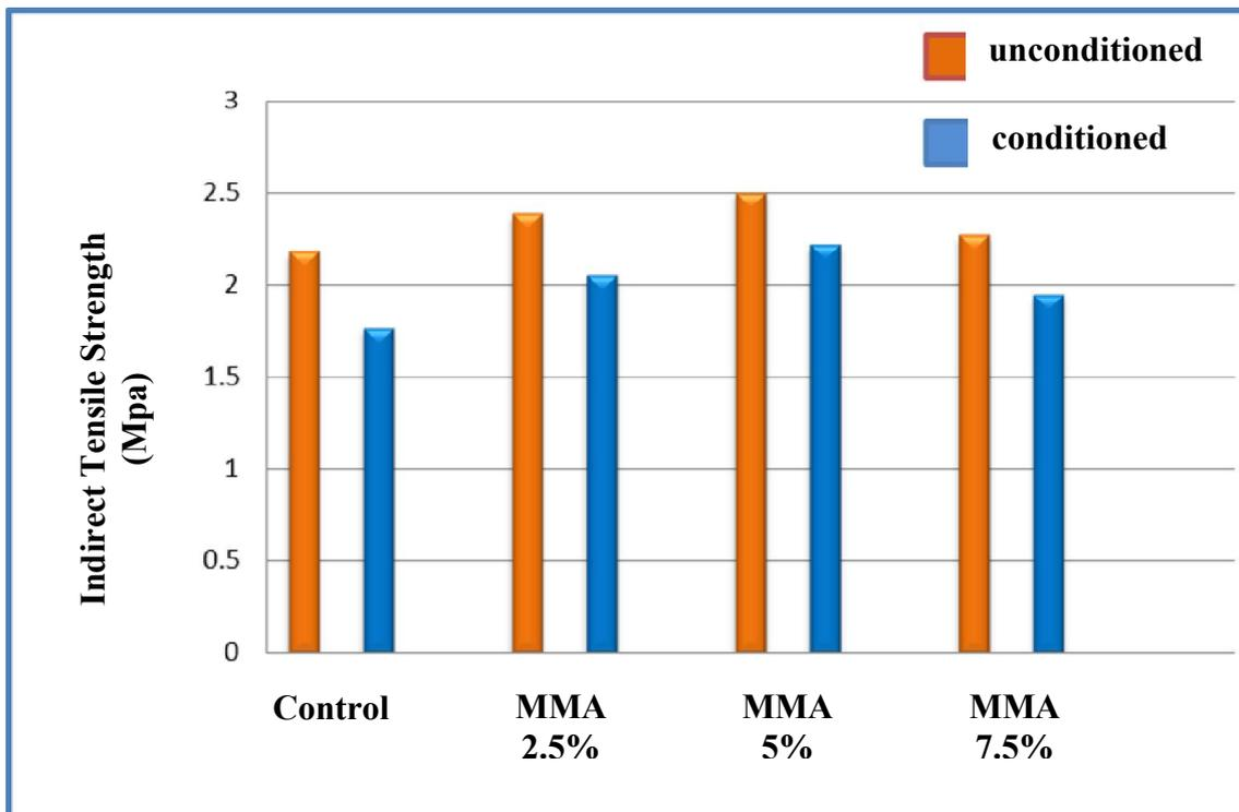
Figure 2: Effect Methyl Methacrylates Polymer (MMA) on the Indirect Tensile Strength (ITS) of Asphalt Concrete Modified Mixture.
