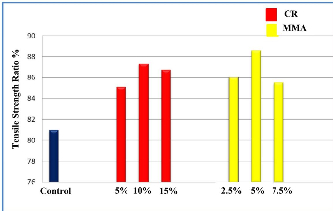
**Figure 3 Effect Crumb Rubber Polymer (CR No 50) and Methyl Methacrylates (MMA) Polymer on the Tensile strength ratio (TSR).**
