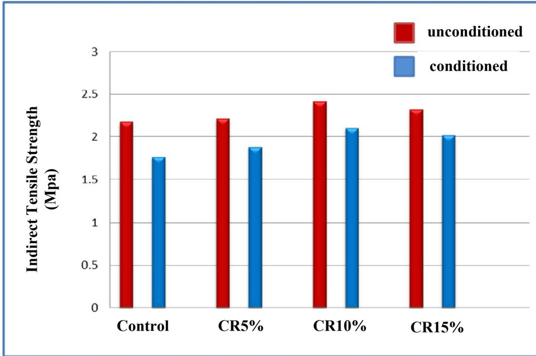
Figure 1: Effect Crumb Rubber Polymer (CR No 50) on the Indirect Tensile Strength (ITS) of Asphalt Concrete Modified Mixture.
