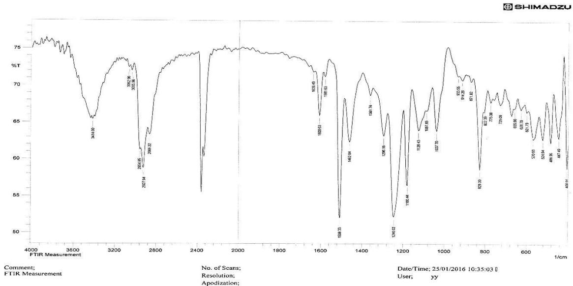
**Figure 3-** FTIR spectrum of epoxy /MWCNTs nanocomposites
