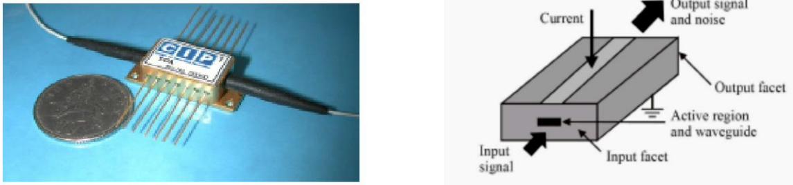
Figure 1: SOA fully packaged (left), and SOA schematic (right) [12].
