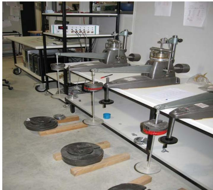
Figure 9: One Dimensional Compression (Oedometer apparatus).
