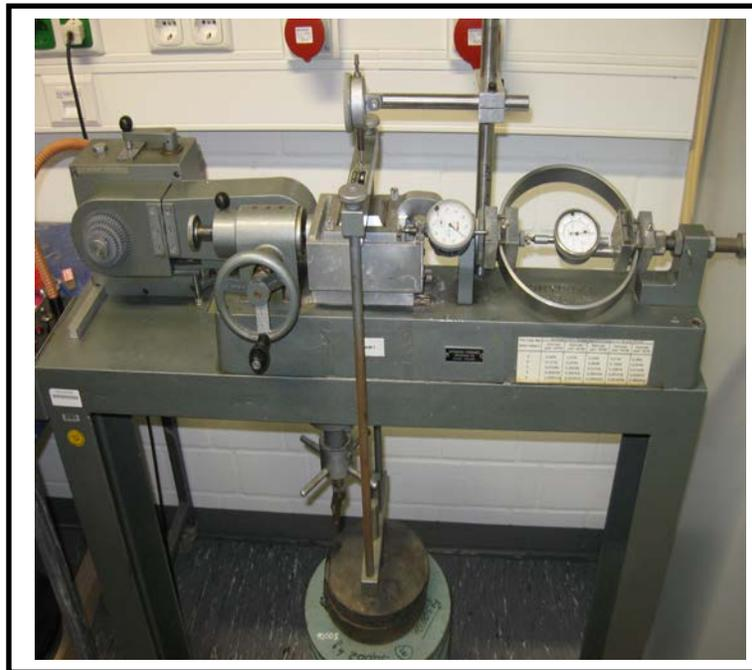
Figure 1: Direct Shear test Apparatus.
