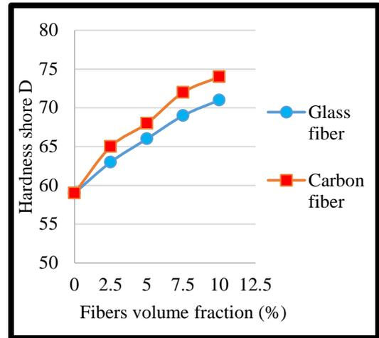
Figure 14: Effect of fibers volume fraction on hardness.
