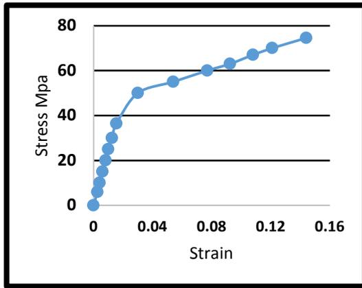
**Figure 6:** The compression stress-strain curve of epoxy resin.
