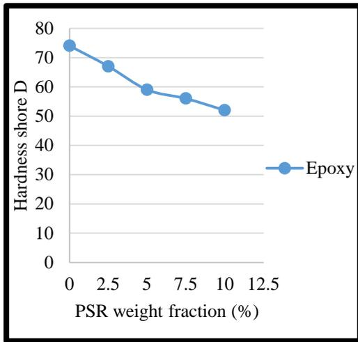
**Figure 10:** Effect of PSR weight fraction on hardness.
