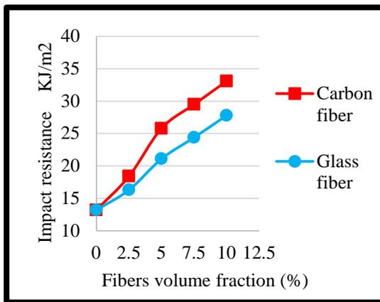
Figure 13: Effect of fibers volume fraction on impact resistance.
