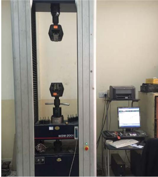
Figure 3: Compression test instrument.
