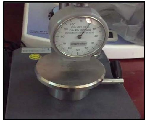
Figure 5: Shore D hardness instrument.
