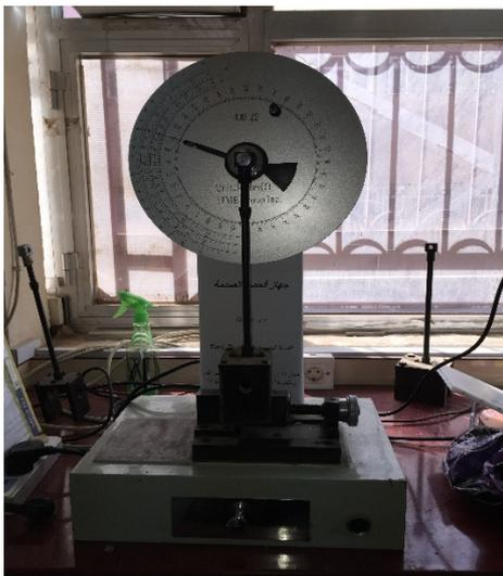
Figure 4: Izod impact test instrument.
