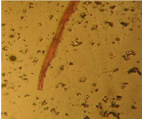
**Figure 4:** shows the distribution homogeneity for reinforcement phases for samples with ratio 7,5% Vf and grain size 25  $\mu\text{m}$  at a magnification of (X800).
