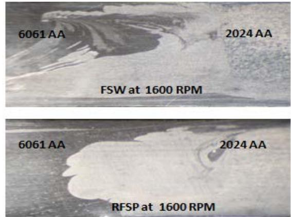
**Figure 10:** Macrostructure, FSW and RFSP
