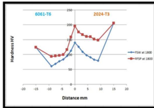
**Figure 14:** Hardness profiles of FSW and RFSP at (1800 RPM, 25 mm/min).
