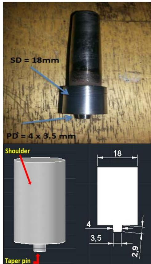
**Figure 4:** FSW, FSP and RFSP tool.
