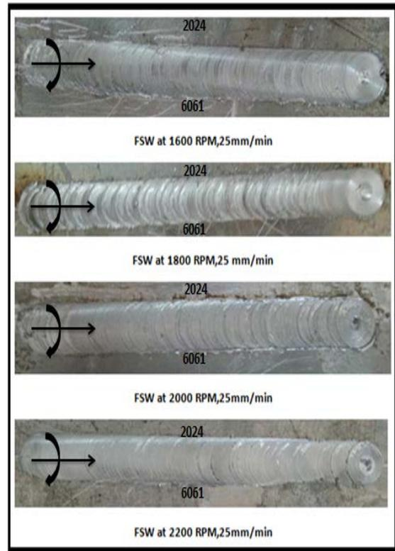
**Figure 6:** surface of welding line for all (FSW) specimens.
