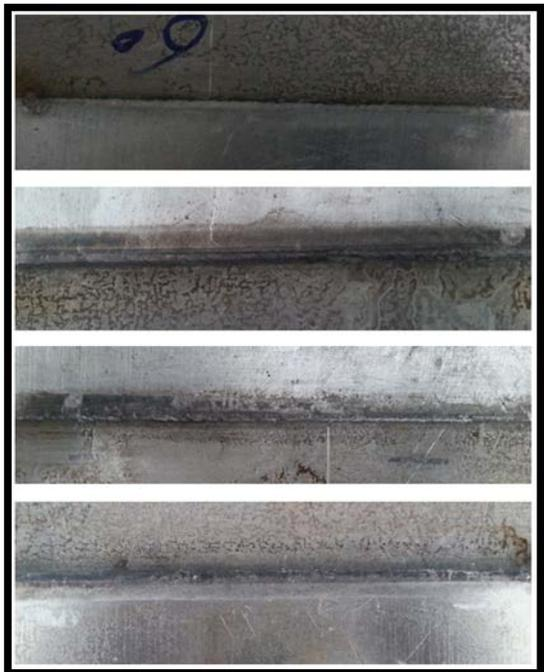
**Figure 8:** The bottom lines of welding for some welded alloys
