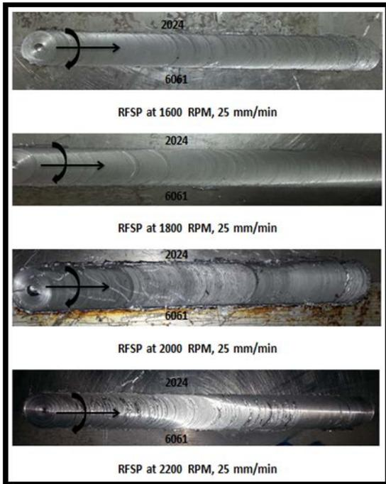
**Figure 7:** surface of welding line for all (RFSP) specimens
