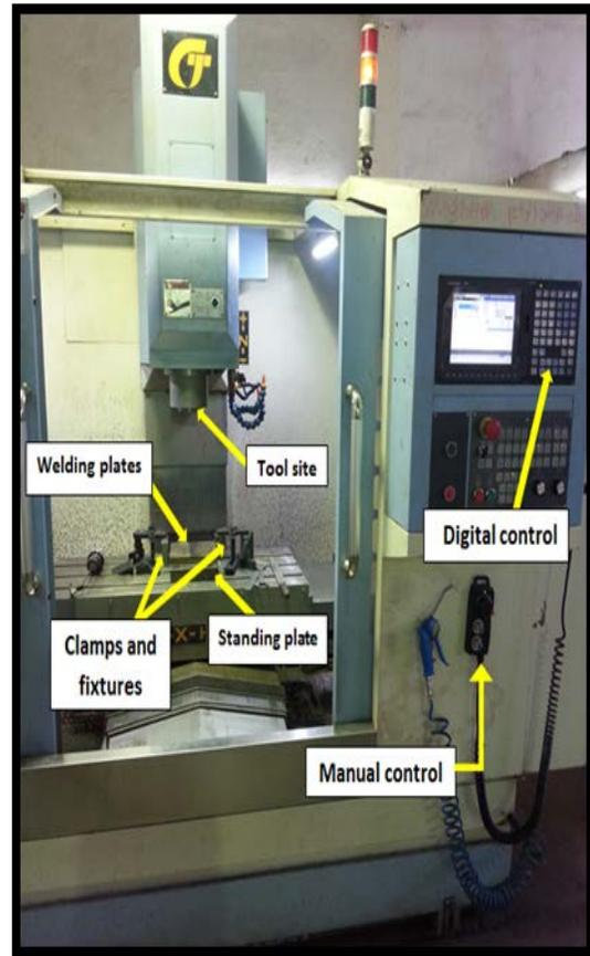
**Figure 2:** MITSUBISHI CNC M70V milling machine.
