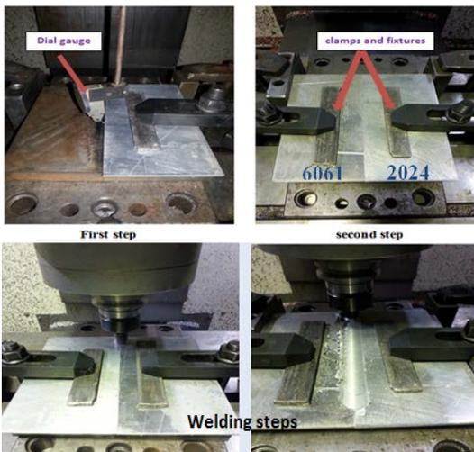
**Figure 3 :** Matching and welding process for two plates.
