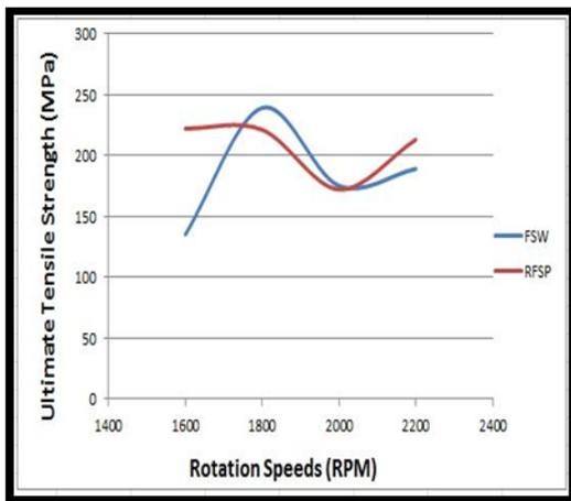
**Figure 9:** Tensile results for FSW and RFSP at different rotation speeds
