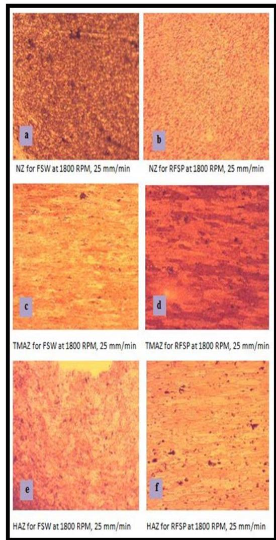
**Figure 11:** The microstructure of the welding zones in FSW and RFSP for dissimilar joints at 1600 RPM, 25 mm/min
