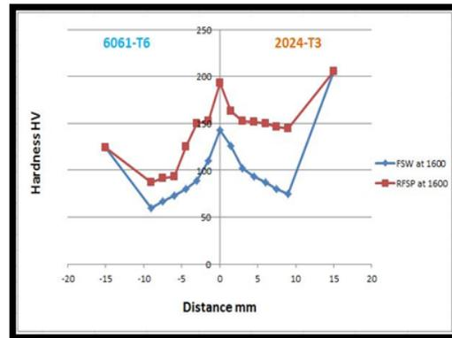
**Figure 13:** Hardness profiles of FSW and RFSP at (1600 RPM, 25 mm/min).
