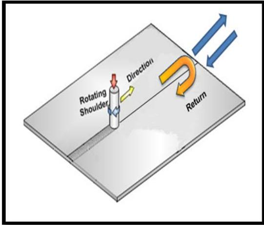
**Figure 1:** Schematic of friction stir processing (FSP) for plates.
