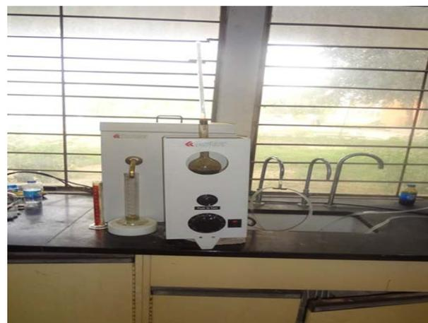
**Figure 1:** Atmospheric distillation unit according to ASTM D -86
