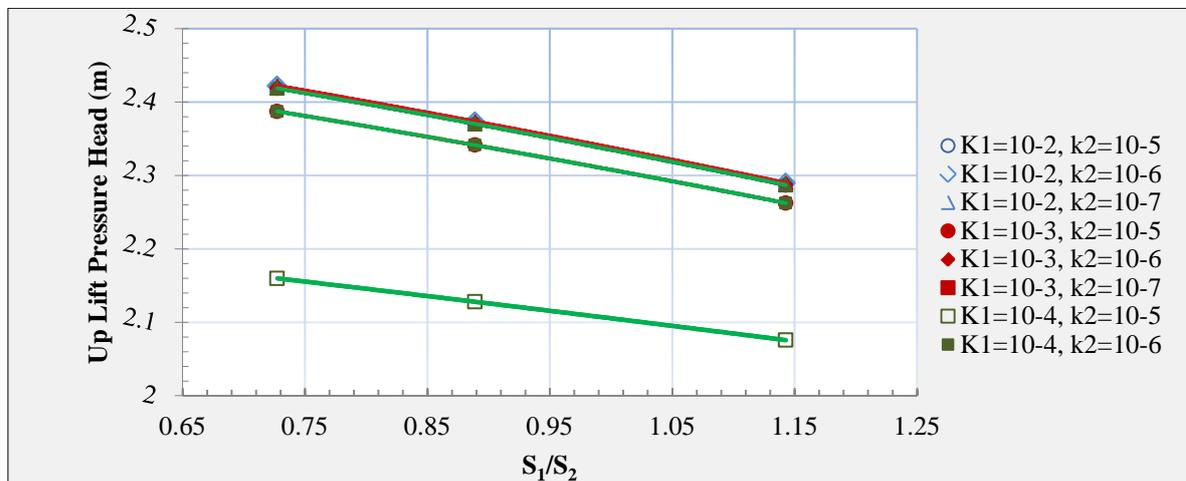
Figure 8: Relationship between Uplift pressure (P) and ( $S_1/S_2$ ) at  $d_1=5.5m$ ,  $d_2=4.5m$  and  $S_1=4m$ .
