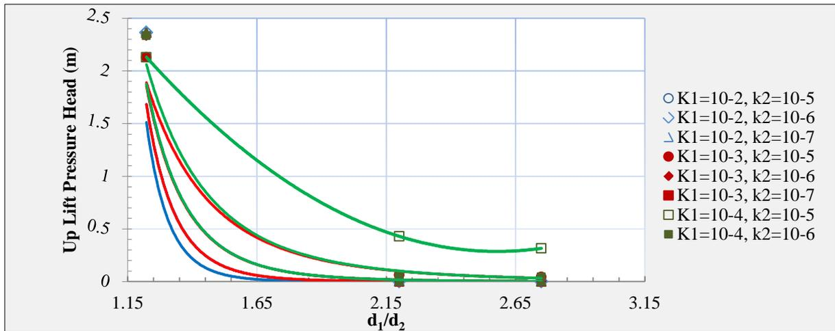
Figure 9: Relationship between uplift pressure (P) and  $(d_1/d_2)$  at  $S_1=3m$ ,  $S_2=3.5m$  and  $d_1=5.5m$
