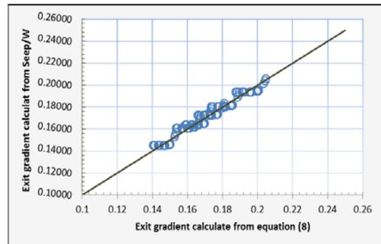
Figure 15: Comparison between the calculated exit gradient from the equation (8) and measuring from SEEP/W model.
