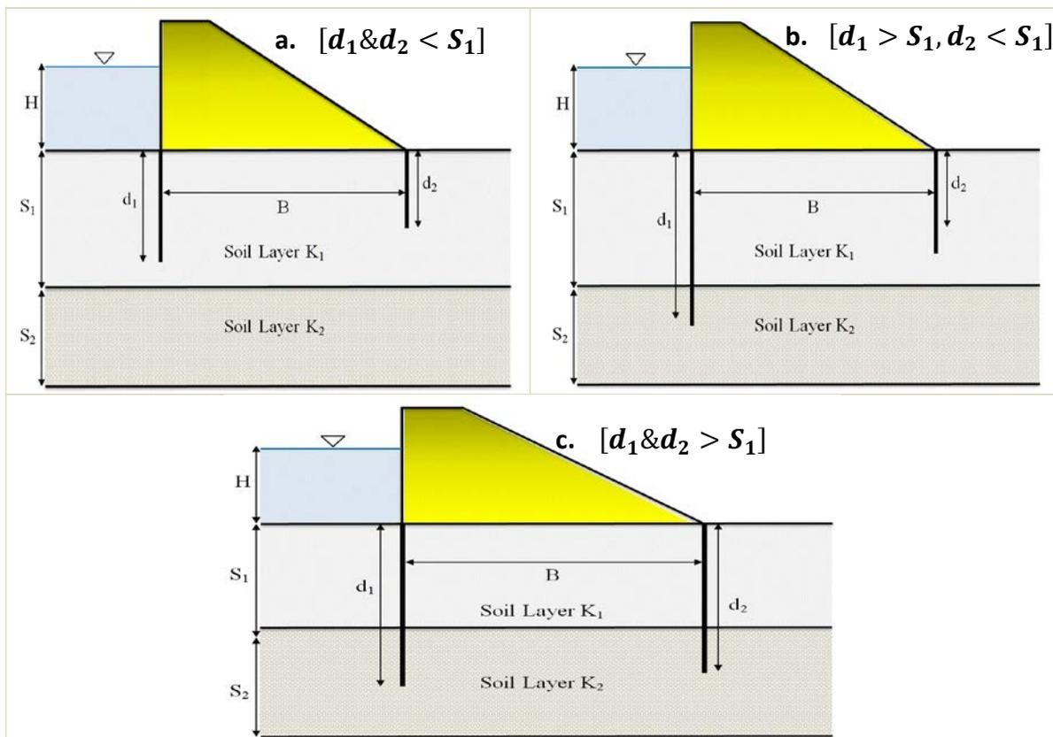
**Figure 2:** The general section of double sheet pile in double soil layer
