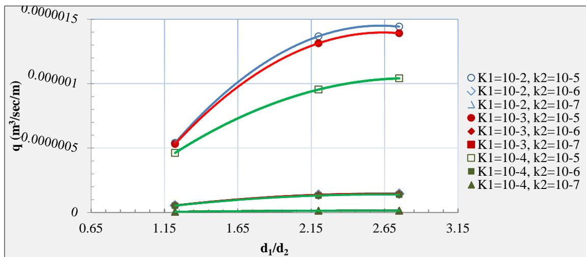
**Figure 6:** Relationship between (q) and ( $d_1/d_2$ ) at  $S_1=3m$ ,  $S_2=3.5m$  and  $d_1=5.5m$ .
