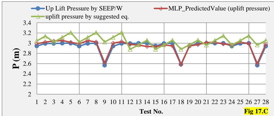
**Figure 17:** Comparison between the calculated exit gradient, discharge and uplift pressure for randomly tests with different method.
