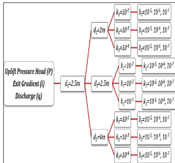
**Figure 1.** The tests for first group ( $d_1=2.5$ m,  $H=6$ m , ( $S_1=3$ )m, ( $S_2=3.5$ )m, ( $b=25$ )m overall first group test (243) run.
