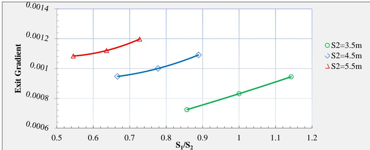
Figure 13: Relationship between exit gradient (i) and  $(S_1/S_2)$  at  $d_1=5.5m$  ,  $d_2=2m$ .
