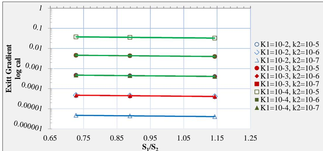
**Figure 11:** Relationship between Exit Gradient (i) and ( $S_1/S_2$ ) at  $d_1=5.5m$ ,  $d_2=4.5m$  and  $S_1=4m$ .
