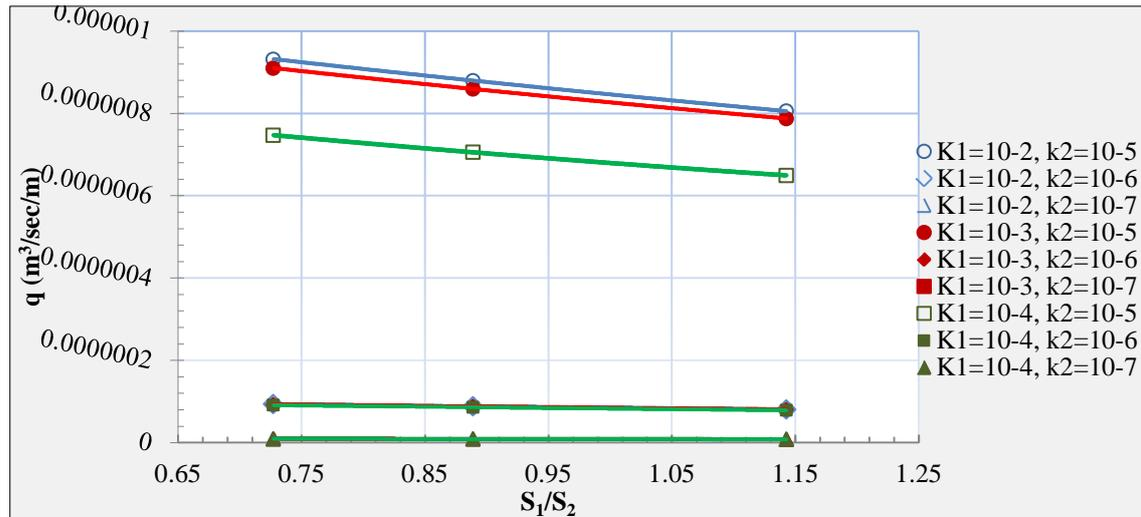
**Figure 5:** Relationship between (q) and ( $S_1/S_2$ ) at  $d_1=5.5m$ ,  $d_2=4.5m$  and  $S_1=4m$
