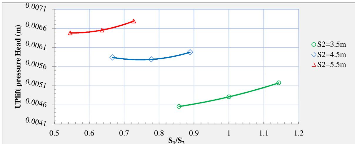
Figure 10: Relationship between (uplift pressure) and  $(S_1/S_2)$  at  $d_1=5.5m$ ,  $d_2=2m$ .
