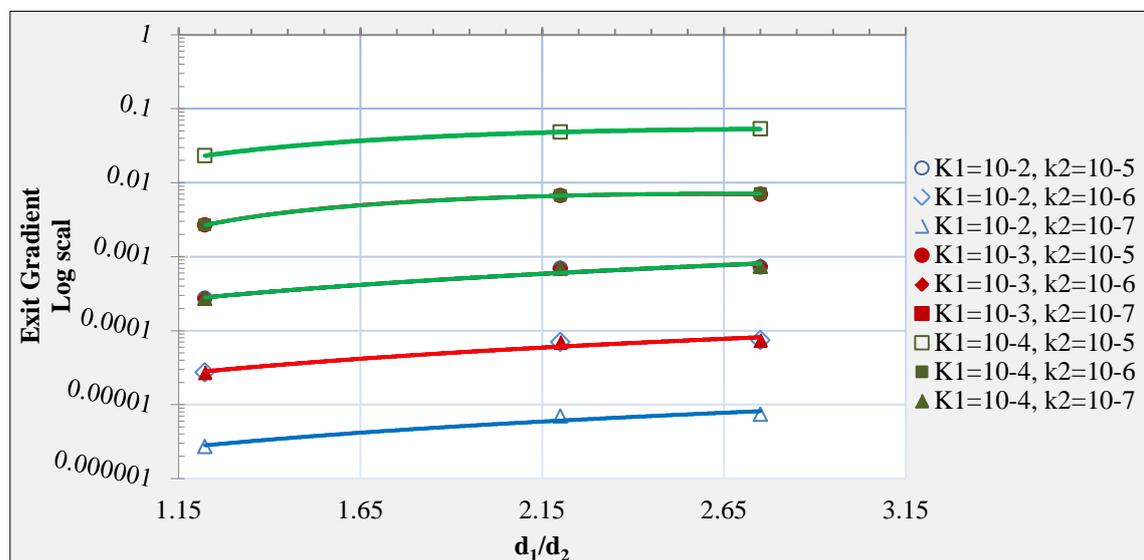
**Figure 12:** Relationship between exit gradient (i) and ( $d_1/d_2$ ) at  $S_1=3m$ ,  $S_2=3.5m$  and  $d_1=5.5m$ .
