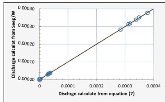
Figure 14: Comparison between the calculated discharge from the equation (7) and those from SEEP/W model.
