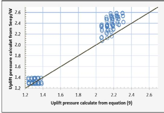
**Figure 16:** Comparison between the calculated uplift pressure from the equation (9) and measuring from SEEP/W model.
