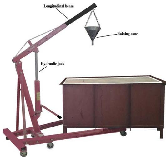
Figure 3: Sand Raining Frame used for controlling density.
