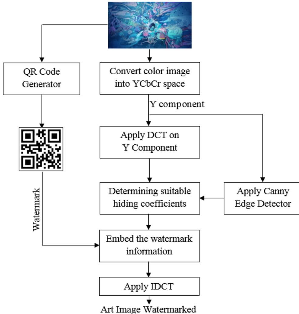
Figure 1: Block diagram of robust watermarking technique for digital art image
