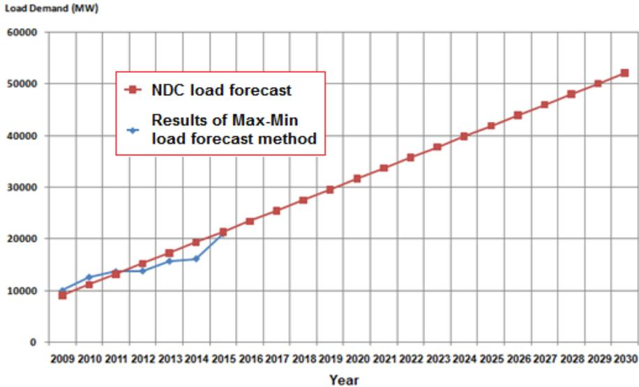
**Figure (5) Load forecast result using Max. - Min. method**
