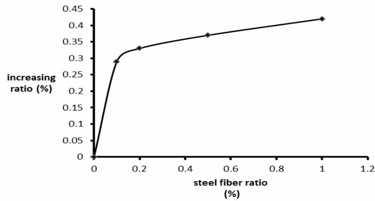
Figure (1): Increasing of compressive strength with various steel fiber ratio.
