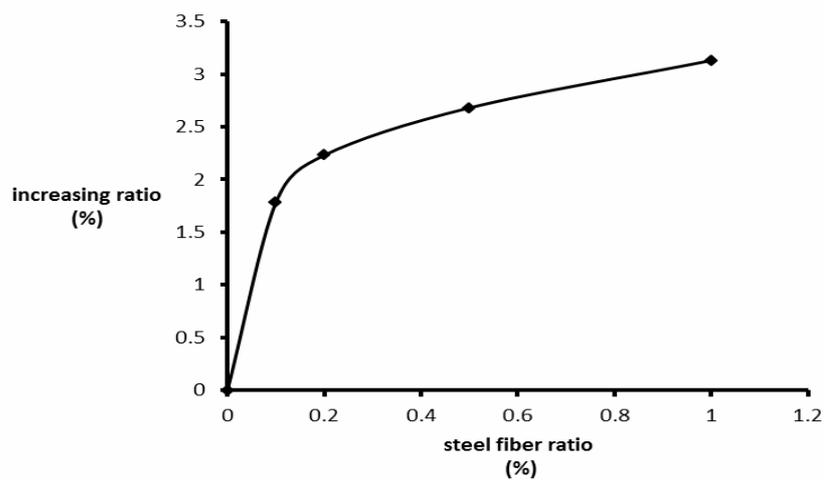
Figure (3): Increasing of flexural strength with various steel fiber ratio.
