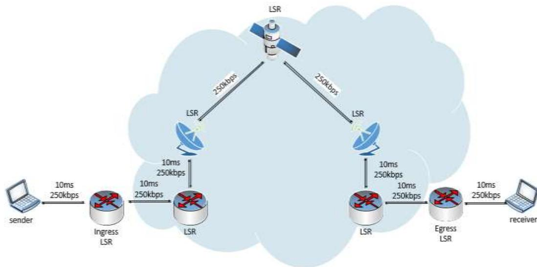
Figure 2- MPLS simulation topology
