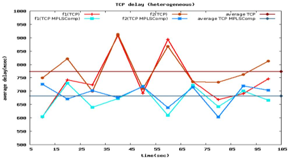
Figure 6-TCP delay for MPLSHCompViaSat using (heterogeneous traffic)
