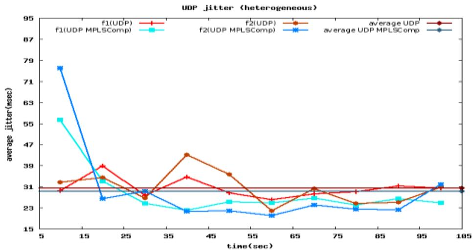
**Figure 9-** UDP jitter for MPLSHCompViaSat using (heterogeneous traffic)
