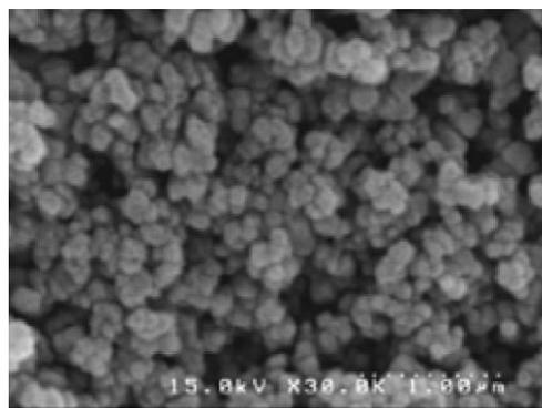
Fig.2. SEM images of TiO<sub>2</sub> nanoparticles.
