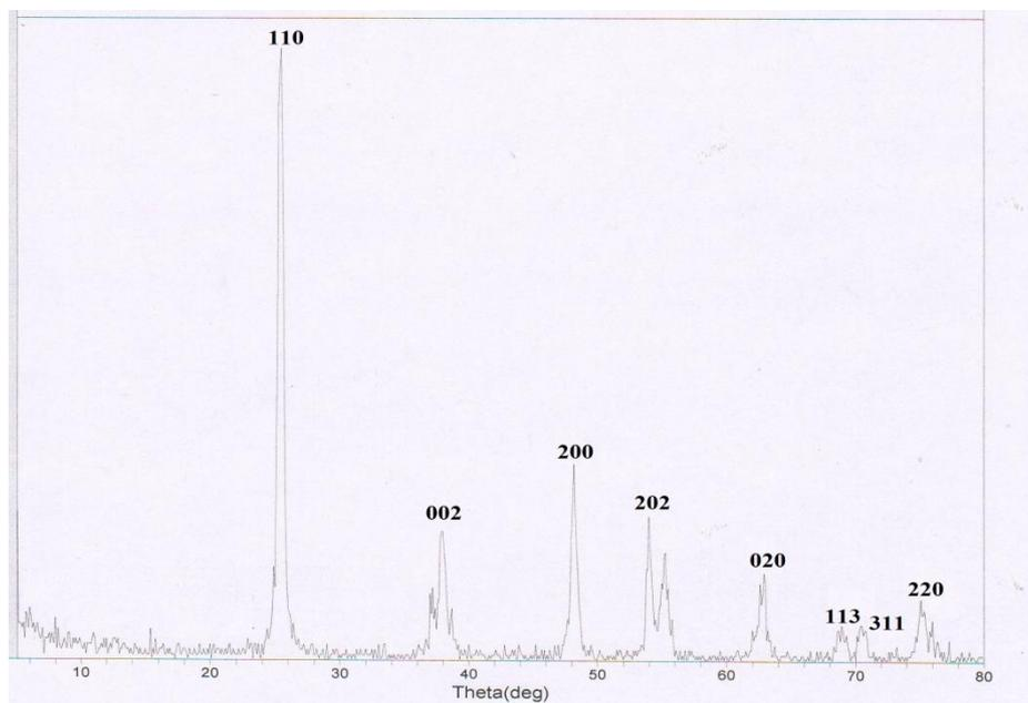
Fig.3. XRD of TiO<sub>2</sub> nanoparticles.
