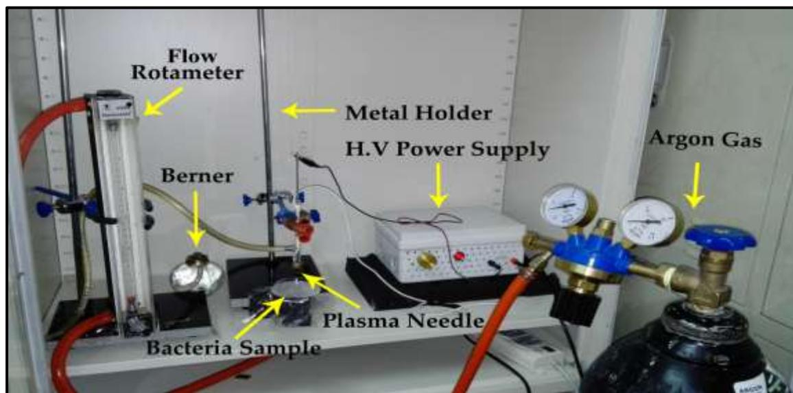
**Figure 2-** the non-thermal plasma needle system.
