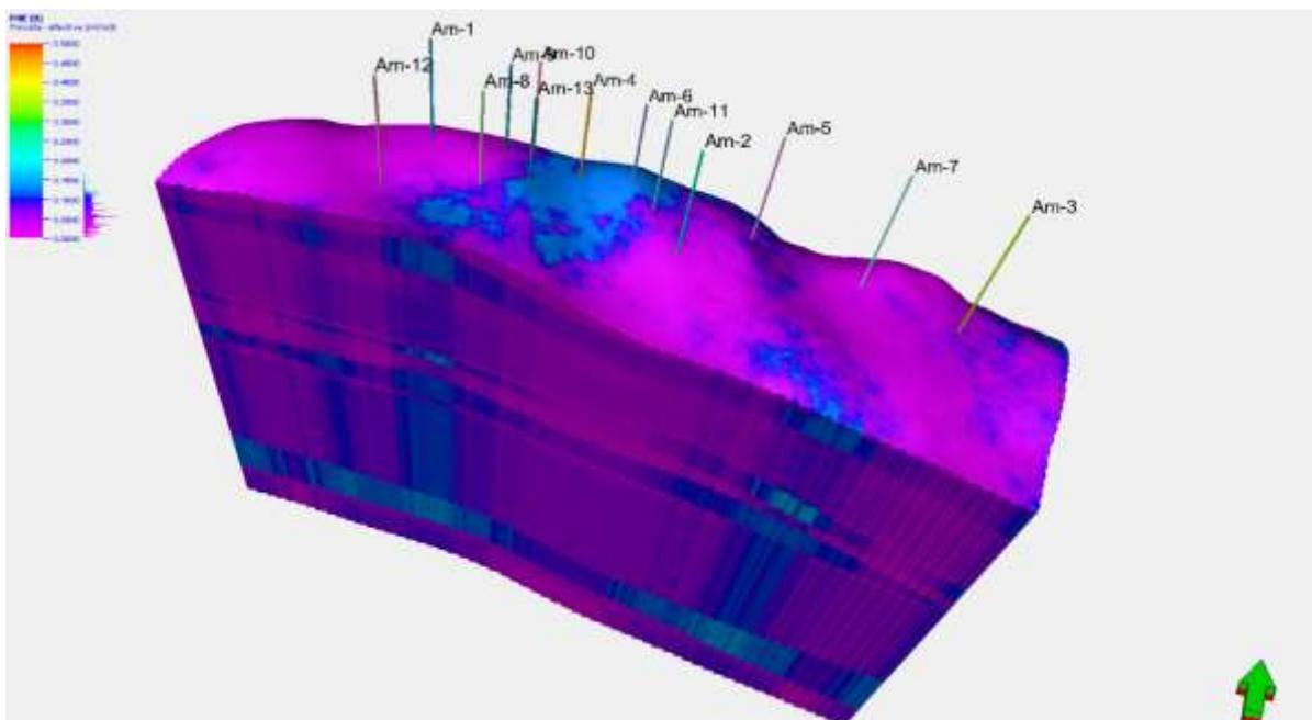
Figure 7- Porosity model of Mishrif Formation in Amara oil field using petrel 2014.
