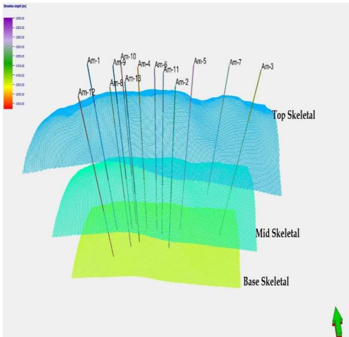
**Figure 5-**The skeletons of Mishrif reservoir in Amara oil field.using petrel 2014.
