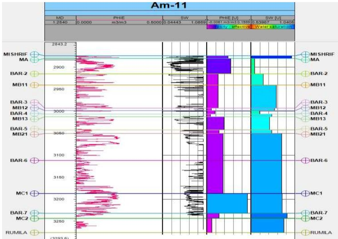
Figure 6- Scale up of porosity and water saturation for Am-11 using petrel 2014
