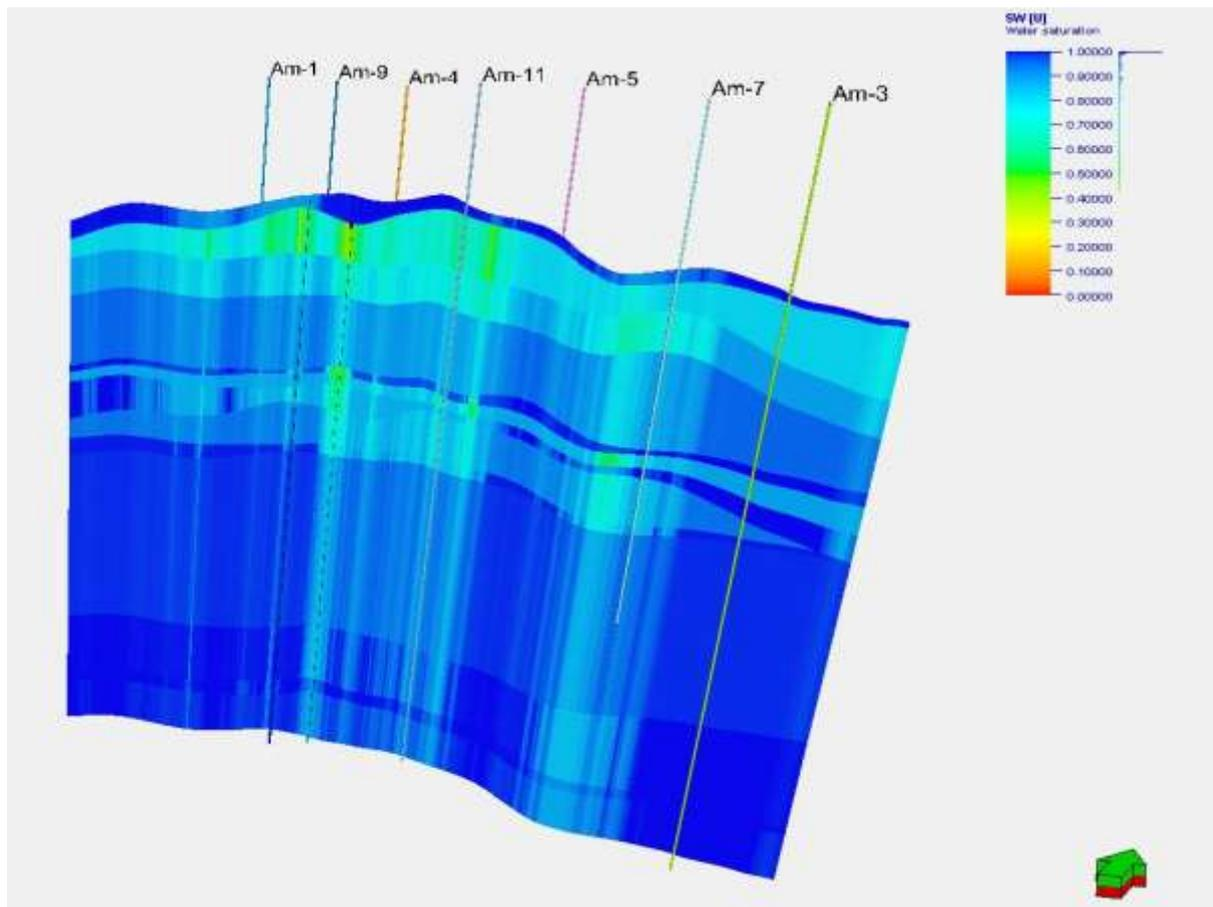
Figure 9- Well section window of Mishrif Formation shows variation in Sw values using petrel 2014.
