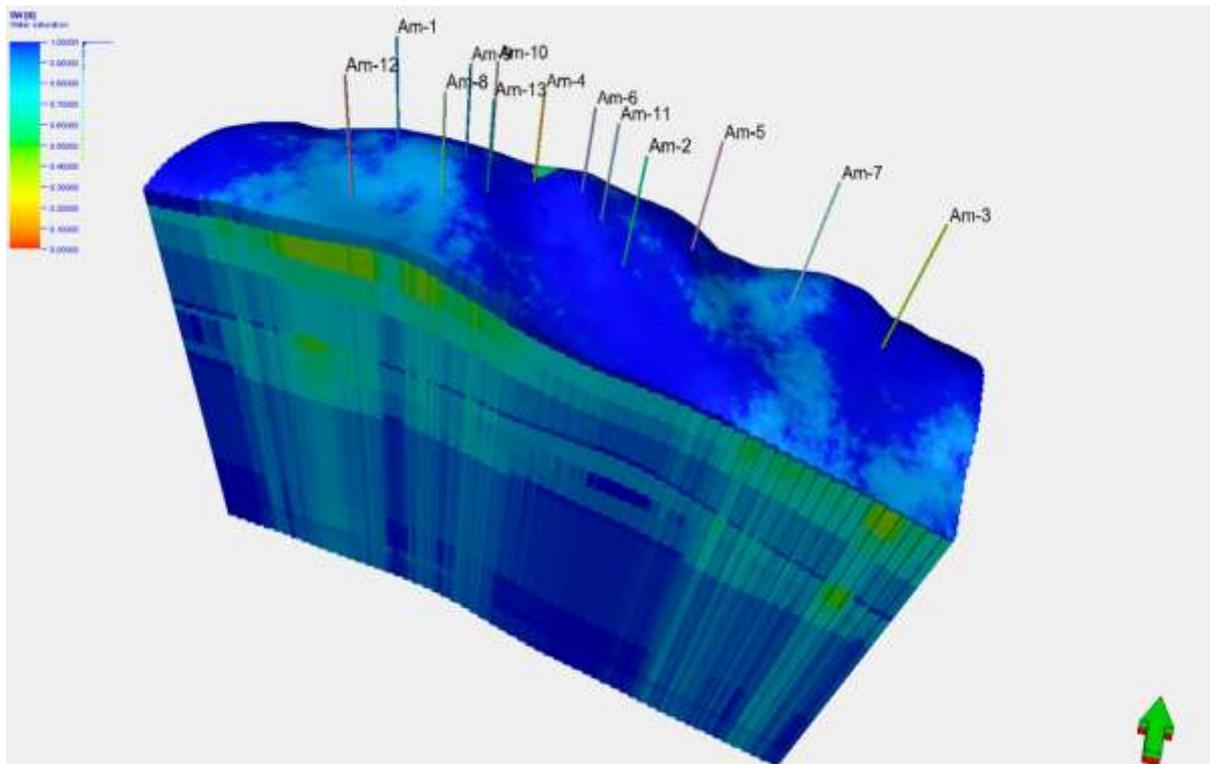
Figure 8- Water saturation model of Mishrif Formation in Amara oil field using petrel 2014.
