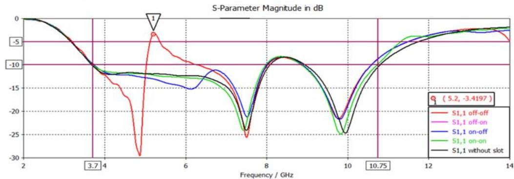
Figure 5: The simulated  $|S_{11}|$  result with varying switching states for the reconfigurable antenna
