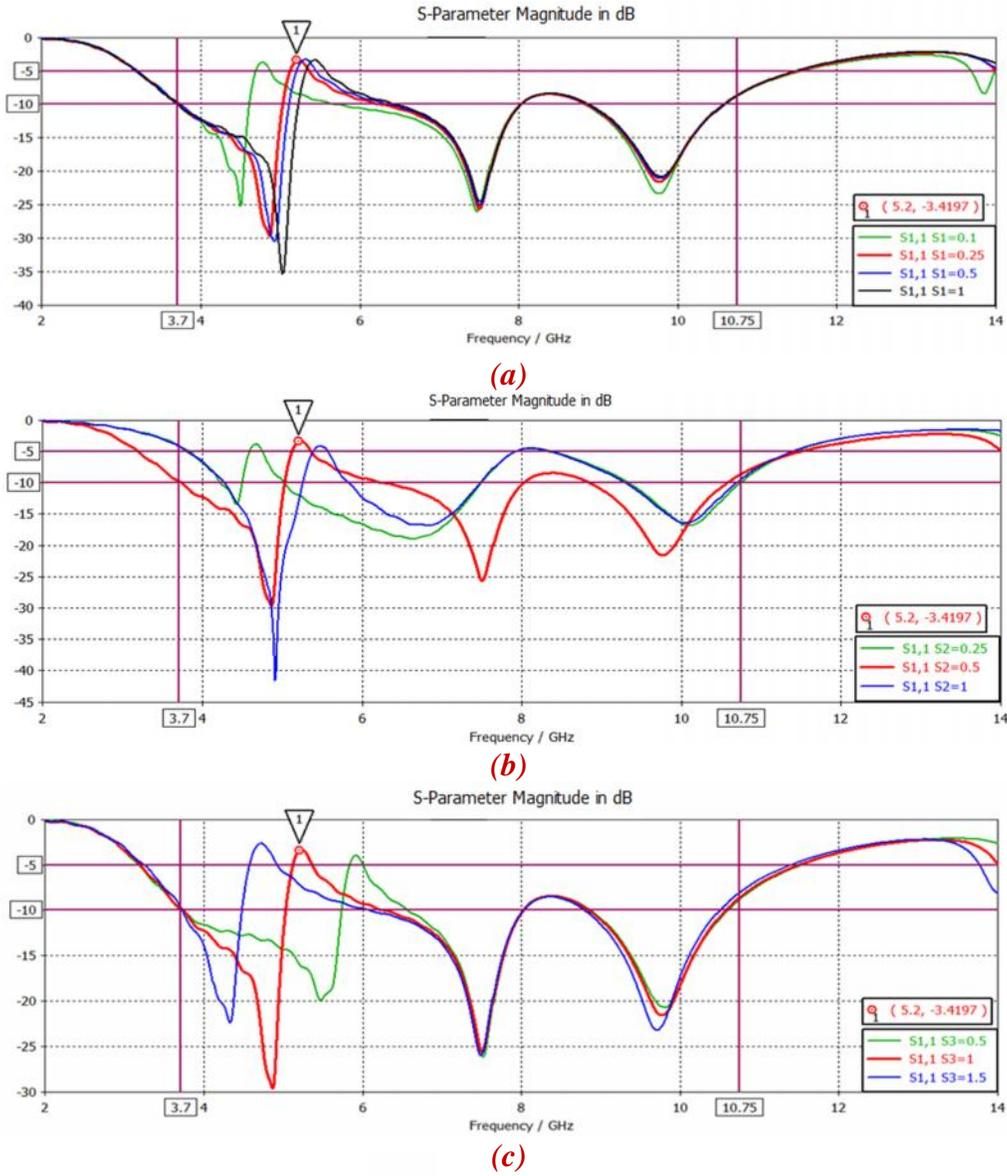
Figure 4: The simulated  $|S_{11}|$  results with a various values to the slot width ( $S_{1,2,3}$ ) parameters for the designed reconfigurable antenna (a)  $S_1$  (b)  $S_2$  (c)  $S_3$
