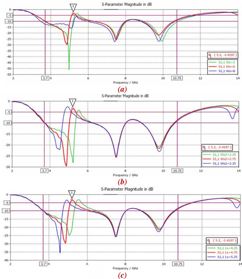
Figure 3: The simulated  $|S_{11}|$  results with a various values to the slot length (WS1,2 and LS) parameters for the designed reconfigurable antenna (a) WS1 (b) WS2 (c) LS
