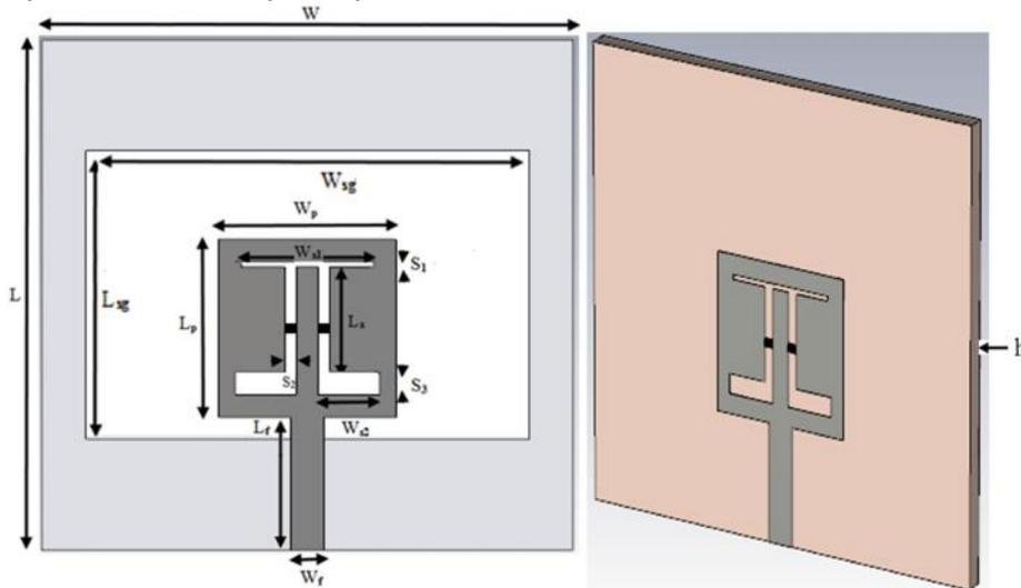
Figure 1: Switchable band notch  $\Gamma$ -slot reconfigurable antenna
