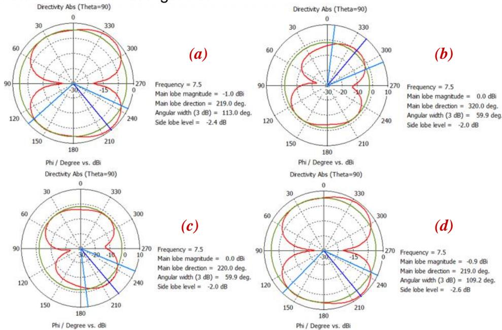
Figure 6: The simulated radiation patterns with varying switching states for the proposed reconfigurable antenna (a) off-off (b) off-on (c) on-off (d) on-on
