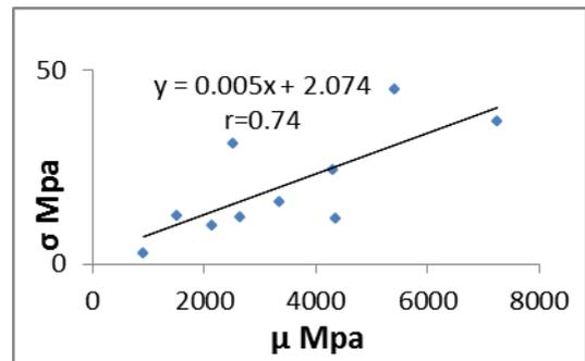
Fig.(8) and (9): Correlation Uniaxial strength with  $k$  and  $\mu$
