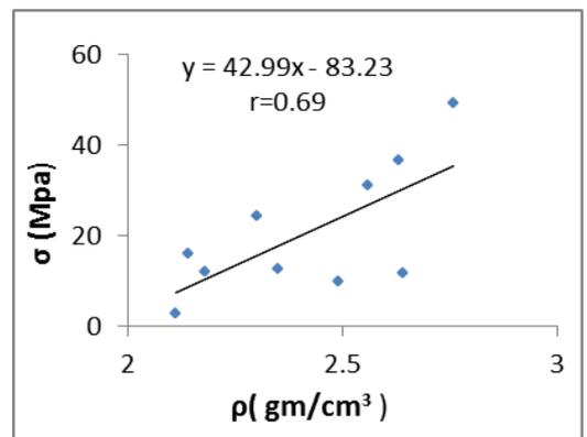
Fig.(10) and (11): Correlation Uniaxial strength with  $E$  and  $\rho$
