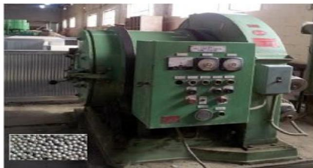
Figure 1. Shot peening device with shot balls
