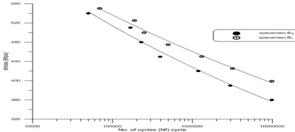
Figure 8. (S-N) curved for low carbon steel (AISI 1010) treatment of surface (B1: shot peening), (B2: laser)
