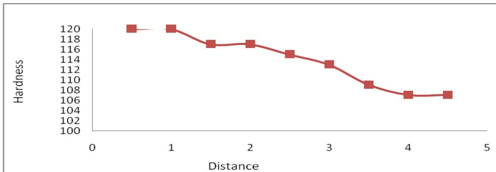
Figure 5. Relationship between the hardness of microscopic samples treated only with laser and the distance from the edge to core
