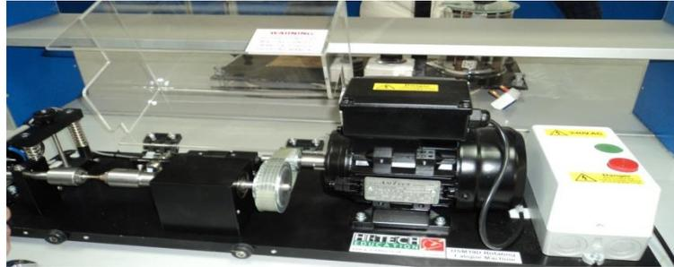
Figure 3. Fatigue testing machine
