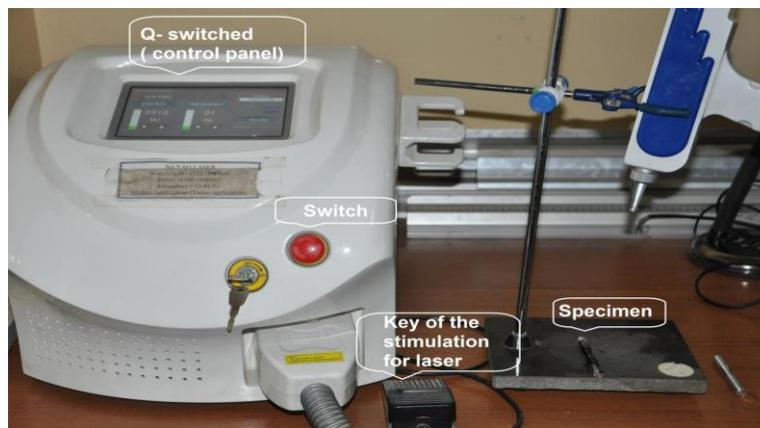
Figure 2. Laser-shock peening
