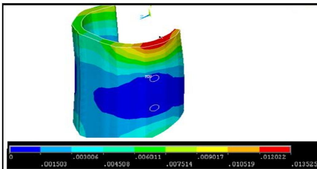
Figure 7. Deformation in elbow made from PCP material ( m )
