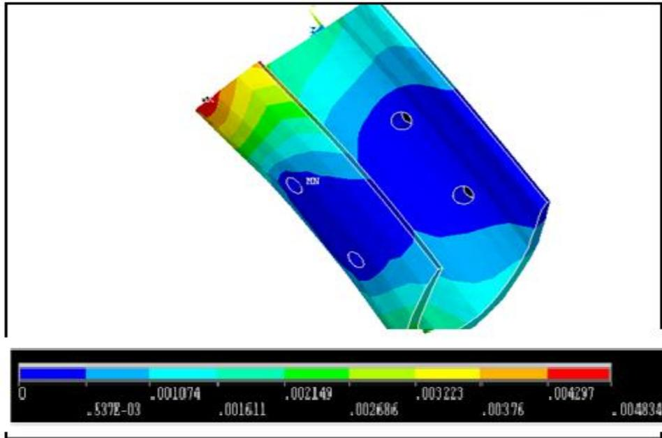
Figure 8. Deformation in elbow made from PP material ( m )
