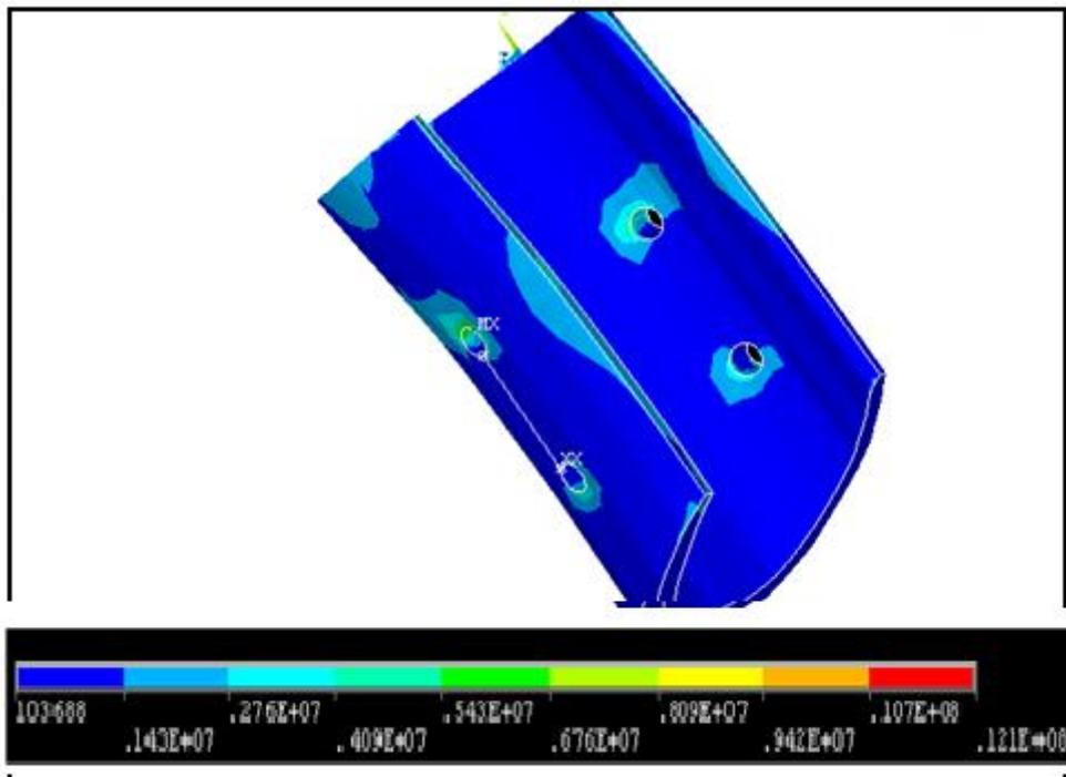
Figure 9. Von – Misses stress in elbow made from PCP material ( N/m<sup>2</sup> )
