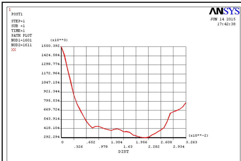
Figure 11. Distribution of Von – Misses stress between holes for PCP material( N/m<sup>2</sup> ).
