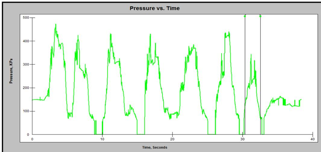
Figure 6. Fluctuating of pressure with time during extension and flexion of elbow ( kPa)
