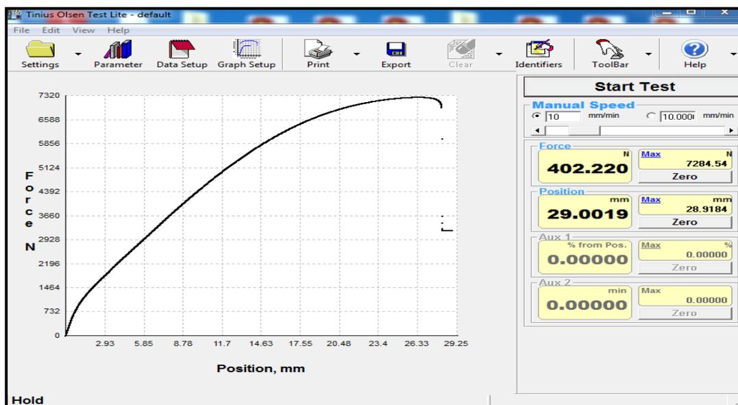
Figure 3. Load – extension chart for PCP material
