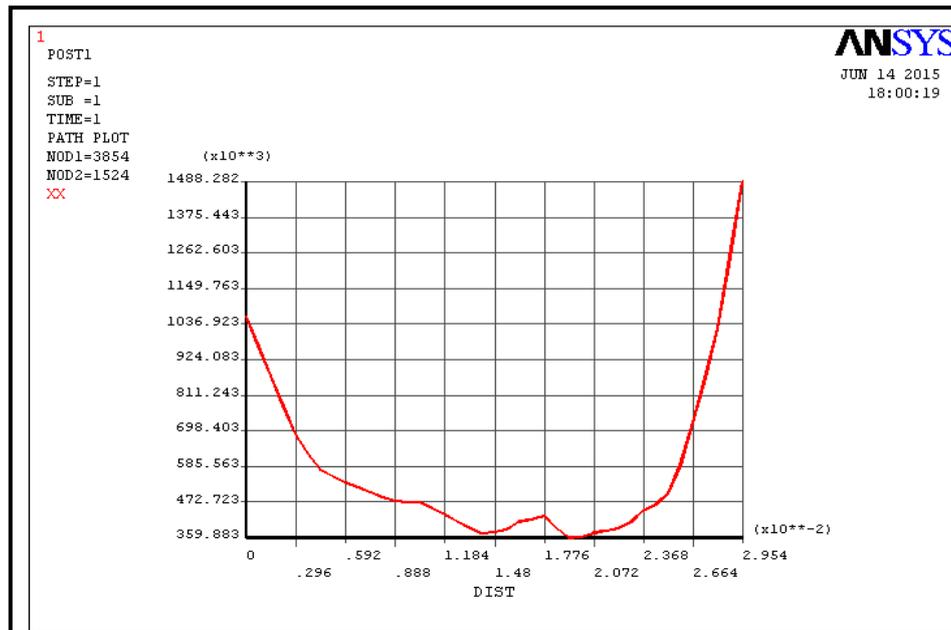
Figure 12. Distribution of Von – Misses stress between holes for PP material(  $\text{N/m}^2$  )
