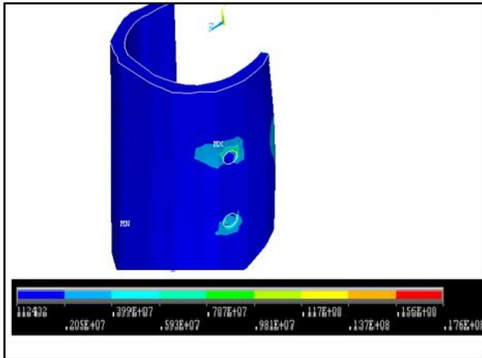
Figure 10. Von – Misses stress in elbow made from PP material ( N/m<sup>2</sup> )
