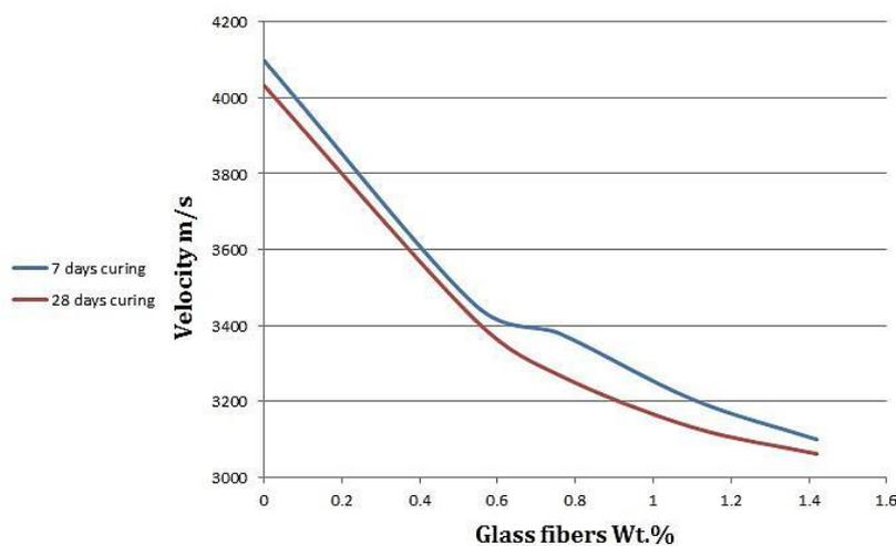
Figure 9. Effect of random glass fibers addition to mortar on velocity
