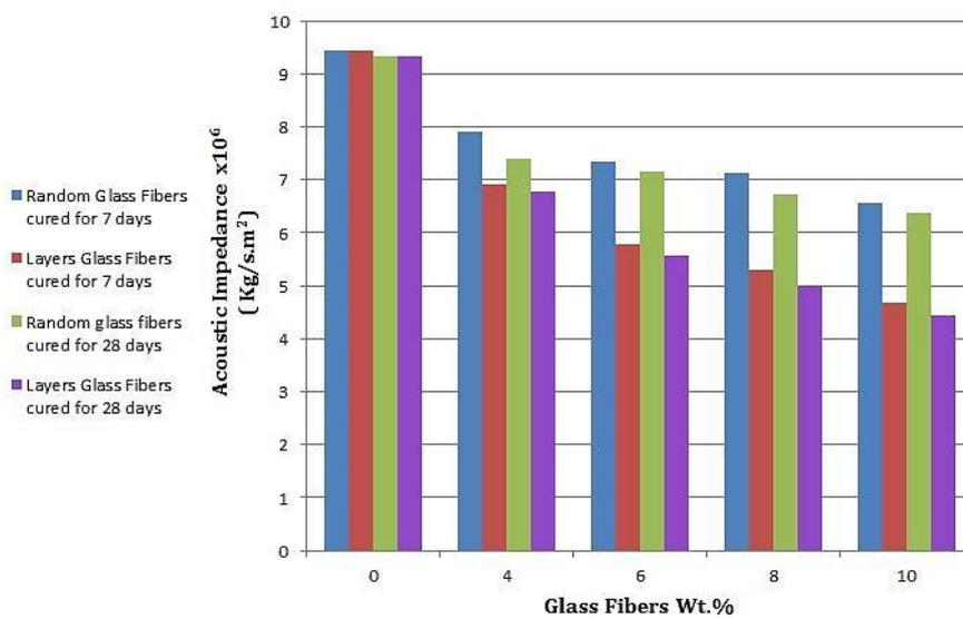
Figure 14. A comparison between the effect of GF (random and layers) addition on the acoustic impedance after 7 and 28 days of curing
