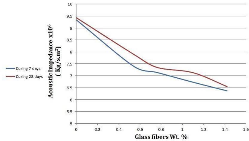
Figure 12. Effect of random glass fibers addition on acoustic impedance
