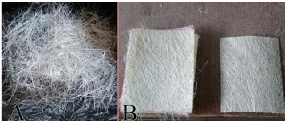
Figure 2. A: Random glass fibers, B: Glass fibers layers.
