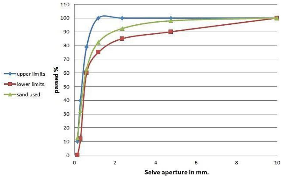
Figure 1. The upper and lower limits of Iraqi specification and the used sand.
