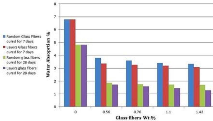
Figure 8. a comparison between the effect of glass fibers on water absorption at 7 and 28 days of curing mortar
