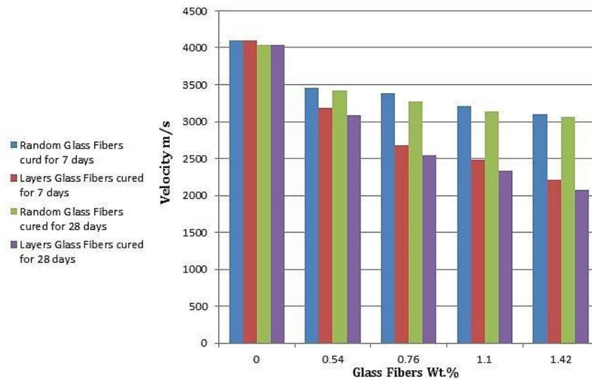
Figure 11. A comparison between the effect of glass fibers (random and layers) addition on the ultrasound wave's velocity after curing for 7 and 28 days
