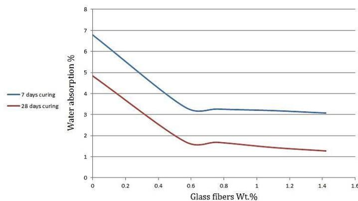
Figure 7. Effect of glass fiber layers addition on the water absorption of mortar
