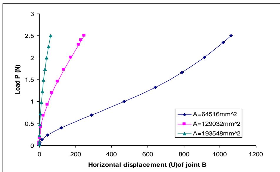
Fig.(17) Effect of cross-sectional area on load-horizontal displacement (U) curve
