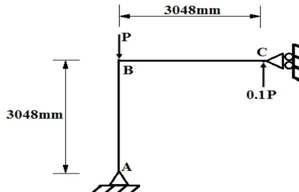
Fig. (32) Geometry and loading of Lee's frame
