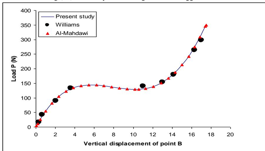
Fig.(27) load - vertical displacement curves at point B for Williams' toggle frame
