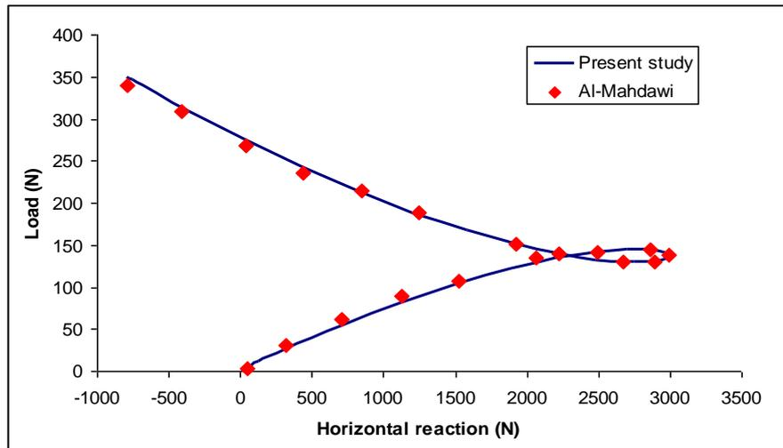
Fig.(28) Load-horizontal reaction curves for Williams' toggle frame
