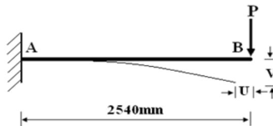
Fig.(11) Geometry and loading of cantilever beam with end load
