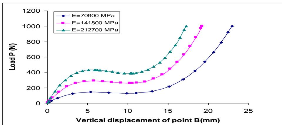
Fig. (31) Effect of modulus of elasticity on load-vertical displacement of point B for Williams' toggle Frame
