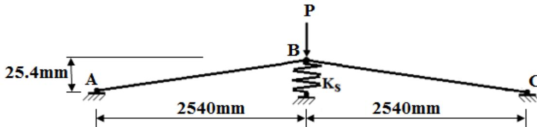
Fig.(7) Geometric and loading of the truss with linear spring
