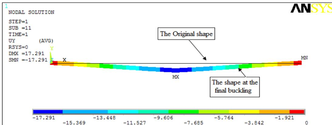
Fig. (23) Variations in vertical displacement for the clamped beam at ultimate load using ANSYS
