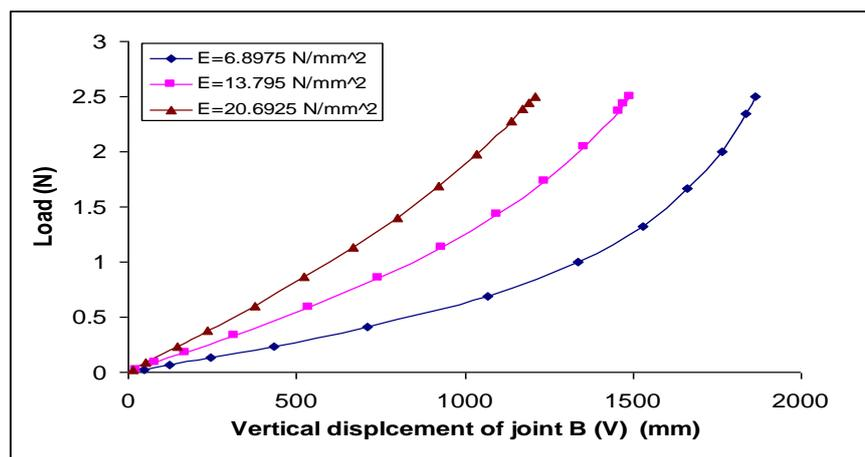
Fig.(18) Effect of modulus of elasticity on vertical displacement (V) curve
