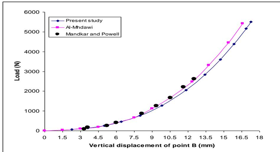
Fig. (22) Load-vertical displacement of joint B of the clamped beam
