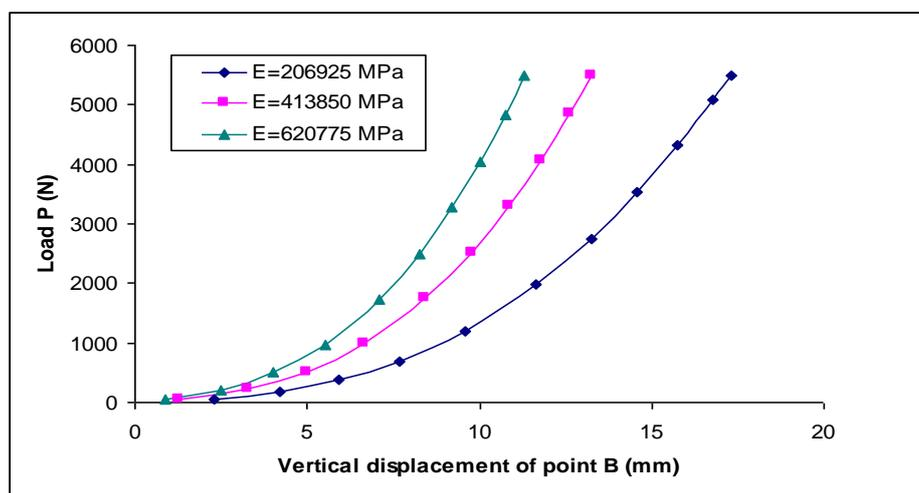
Fig.(25) Effect of modulus of elasticity on load-vertical displacement of joint B of clamped beam
