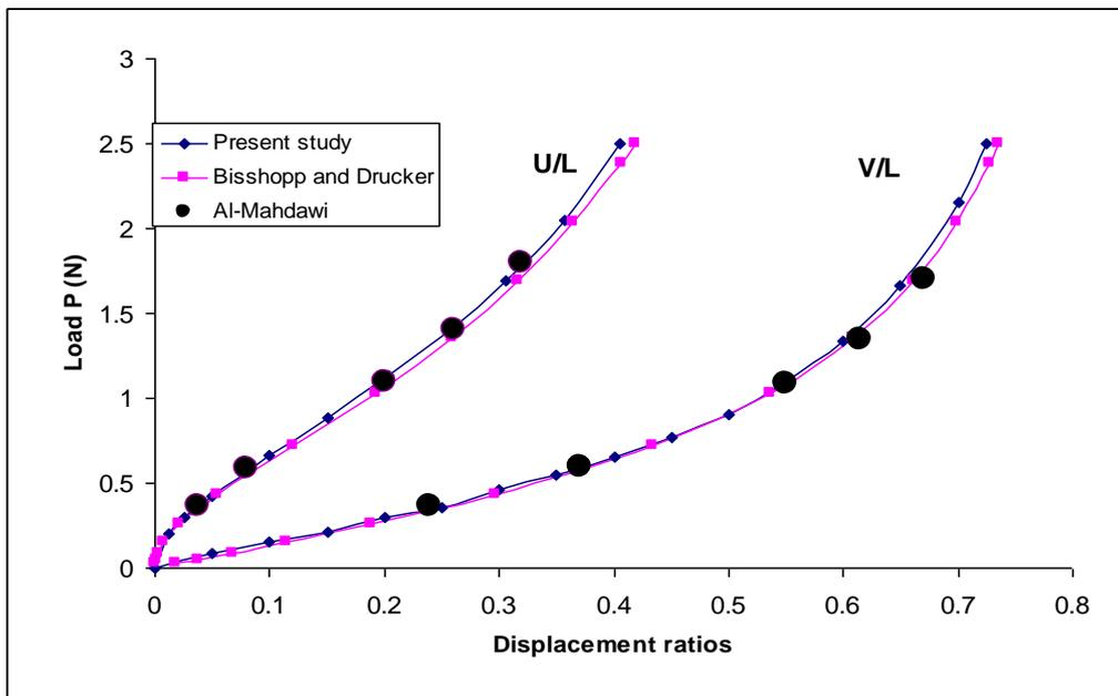
Fig.(14) Load-vertical and horizontal displacement curves of cantilever beam with end load
