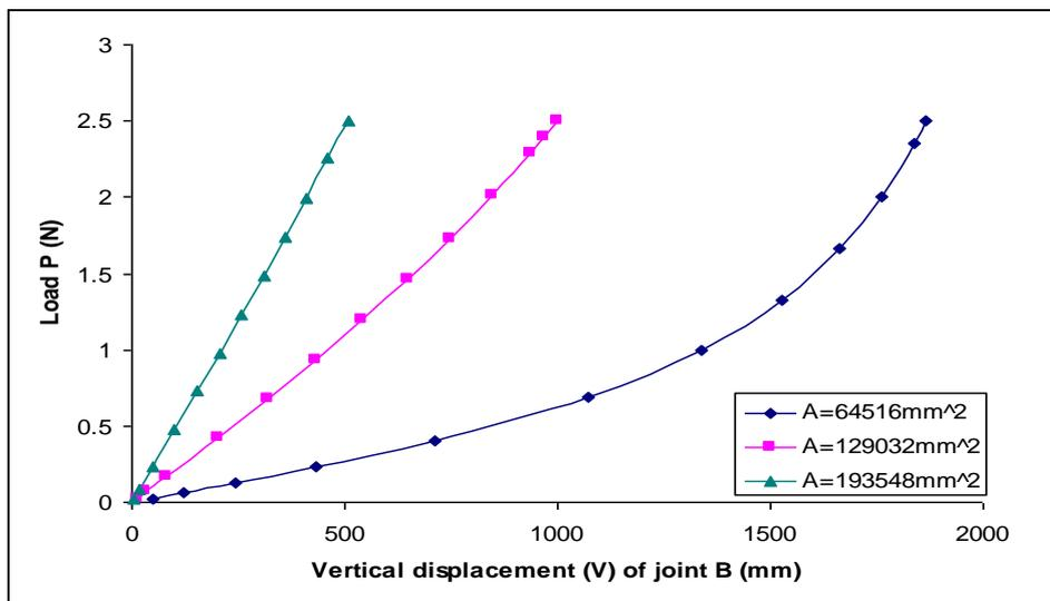
Fig.(16) Effect of cross-sectional area on load-vertical displacement (V) curve
