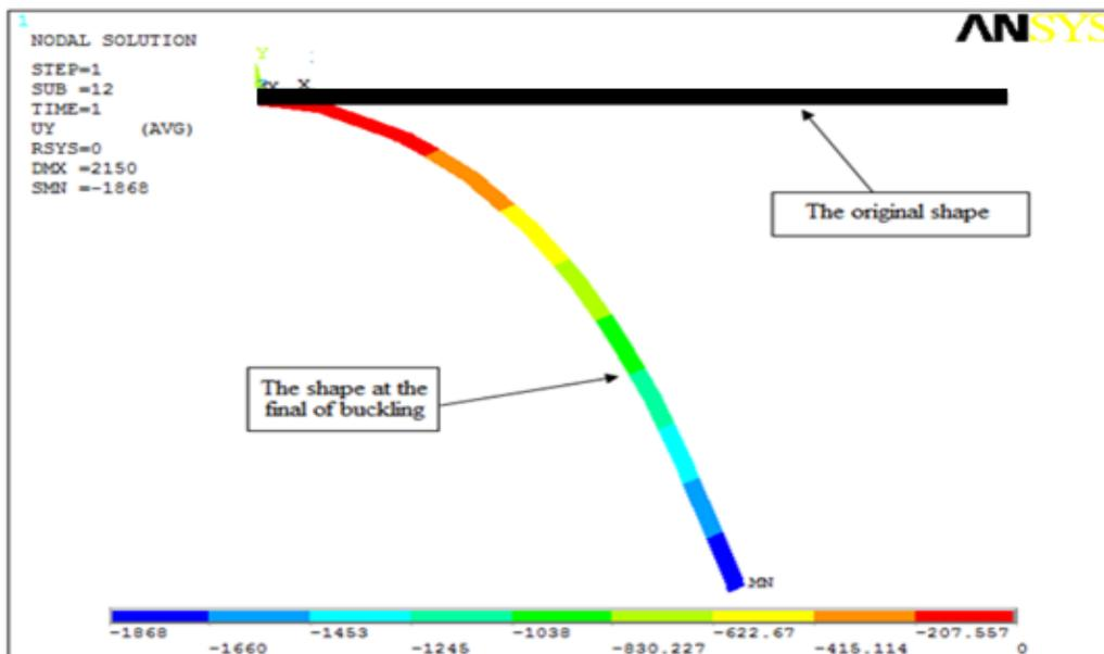
Fig. (15) Variations in vertical and horizontal displacement for the cantilever beam at ultimate load using ANSYS
