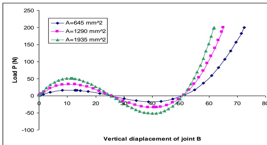
Fig.(10) Effect of cross sectional area on load-displacement curve of two bar truss
