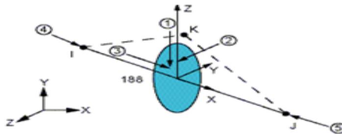
Fig.(12) Geometry of BEAM188 element [13]
