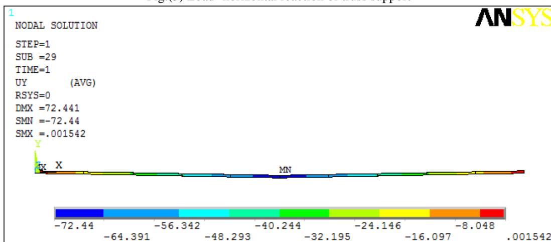
Fig.(6) Variations in vertical displacement for the truss at ultimate load using ANSYS
