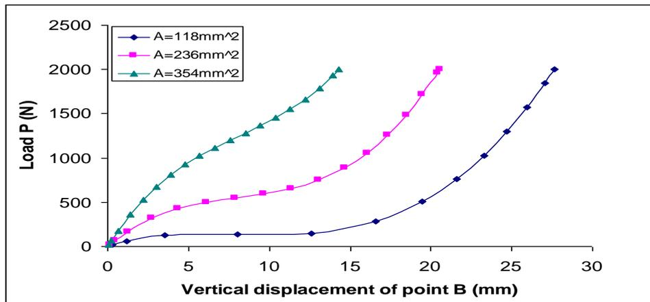
Fig.(30) Effect of cross-sectional area on load-vertical displacement of point B for Williams' toggle Frame
