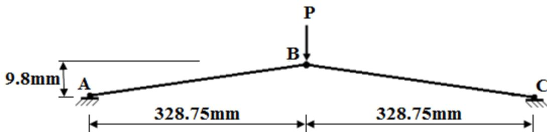
Fig.(26) Geometry and loading Williams' toggle frame
