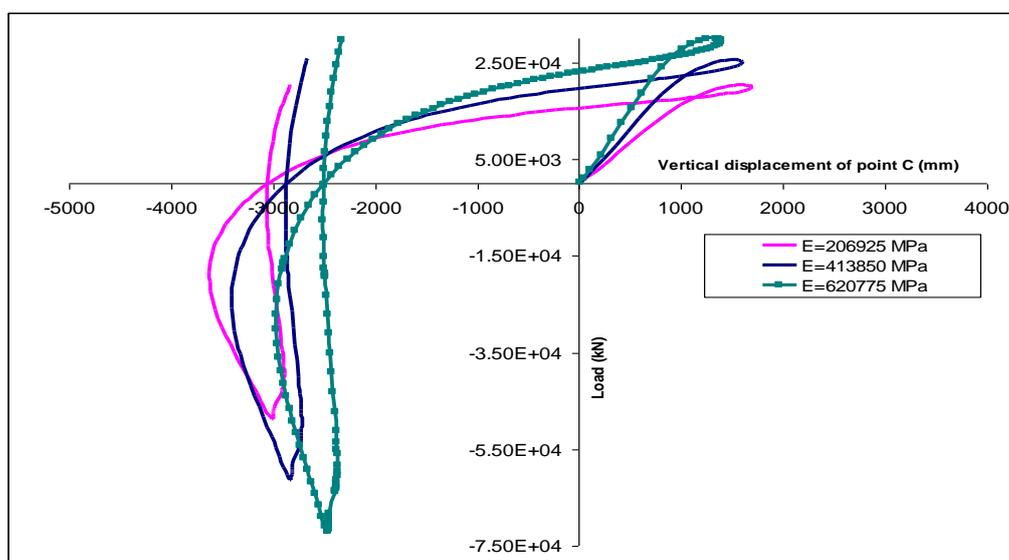
Fig. (37) Effect modulus of elasticity on load-vertical displacement of point C for Lee's frame
