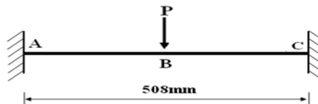
Fig.(20) Geometry and loading of clamped beam
