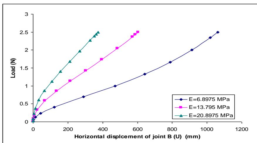
Fig.(19) Effect of modulus of elasticity on horizontal displacement (U) curve
