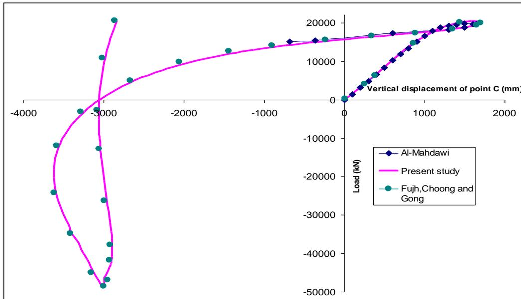
Fig.(34) Load-vertical displacement of point C for lee's frame
