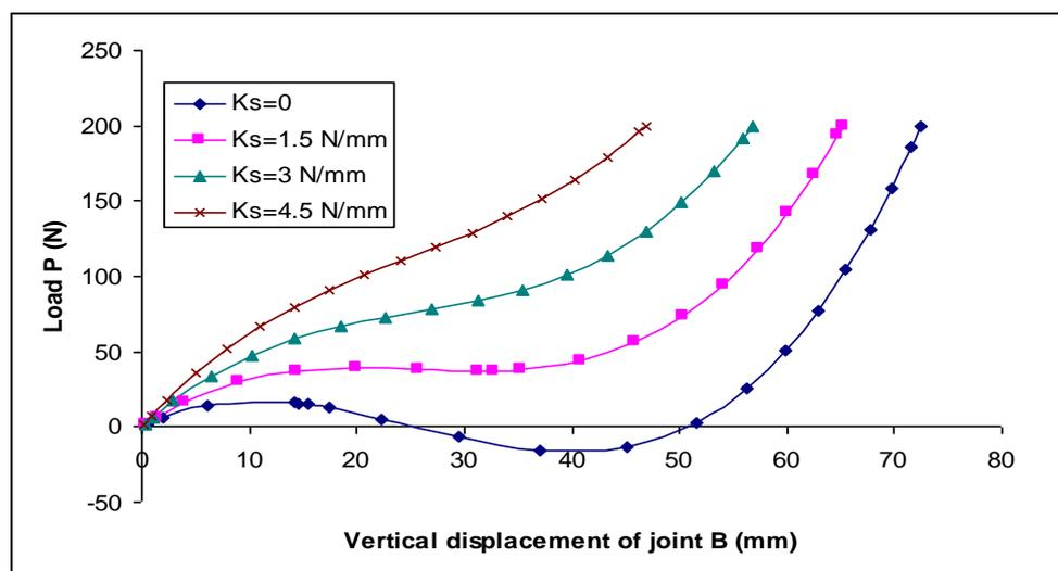
Fig.(9)Effect of linear spring stiffness on load-displacement curve of two bar truss
