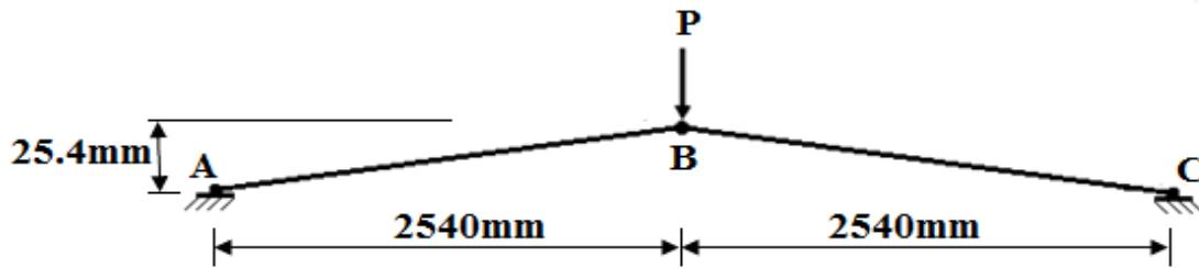
Fig.(1) Geometry and loading of two bar truss
