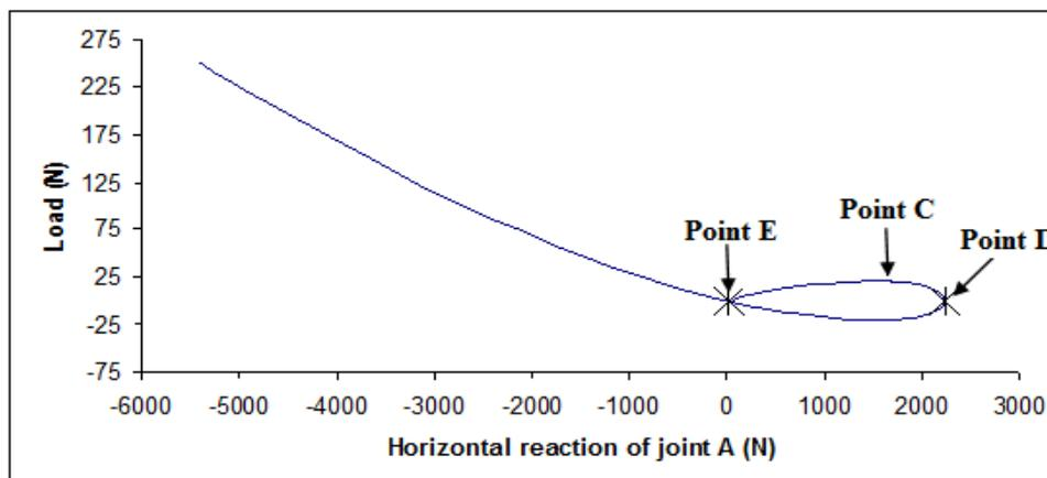
Fig.(5) Load- horizontal reaction of truss support
