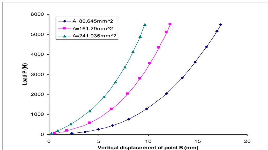
Fig.(24) Effect of cross-sectional area on load-vertical displacement of joint B of clamped beam
