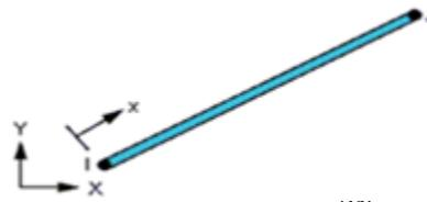
Fig.(2) LINK1 element <sup>[13]</sup>
