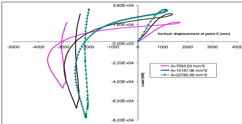
Fig. (36) Effect cross-sectional area on load-vertical displacement of point C for Lee's frame
