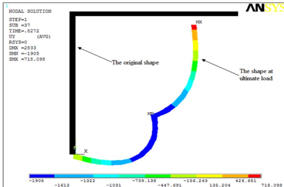
Fig. (35) Variations in vertical displacement for lee's frame at ultimate load using ANSYS
