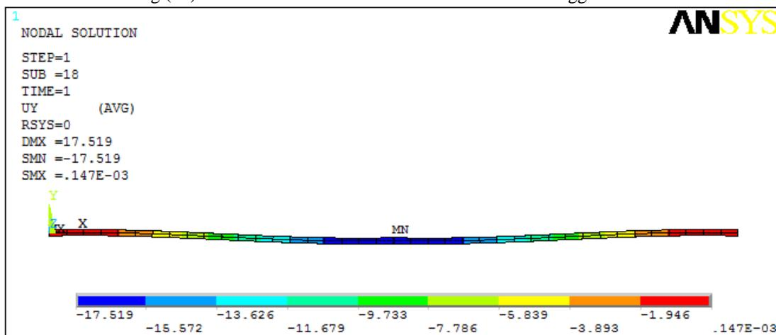
Fig.(29) Variations in vertical displacement for the Williams' toggle frame at ultimate load using ANSYS
