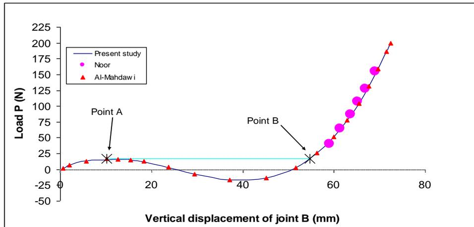
Fig.(4) load-displacement curve of two bar truss
