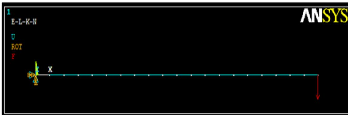
Fig.(13) Modeling the cantilever beam in ANSYS
