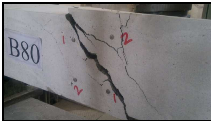
Figure (14), Crack Pattern and Failure Mode of High Strength SCC Beam (B80)
