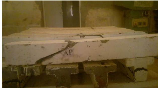
Figure (7), Failure Mode of Normal Strength SCC Beam (Ap)
