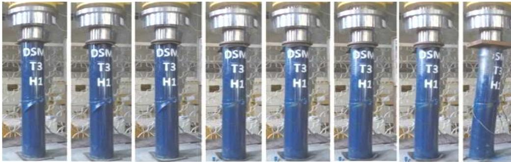
c) CFDSST Specimen no. (3), labeled as (DSM-T3-H1)
