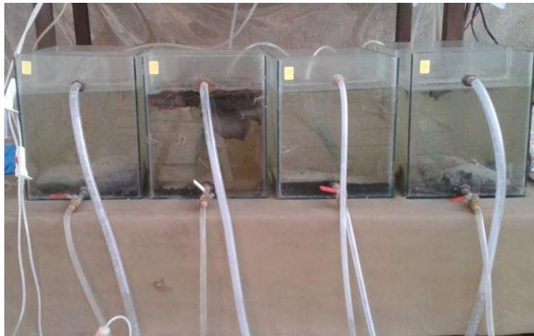
Figure 6. Side view of the FC showing rising sludge and septic conditions
