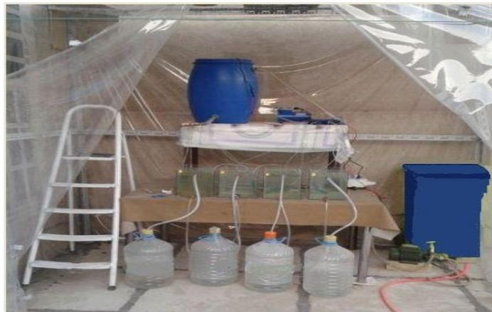
Figure 2: The experimental setup of the biological reactor
