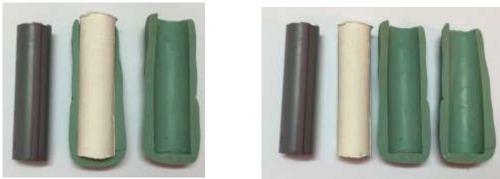
Fig. (1):Plastic pattern, plaster sample and silicone putty mould
