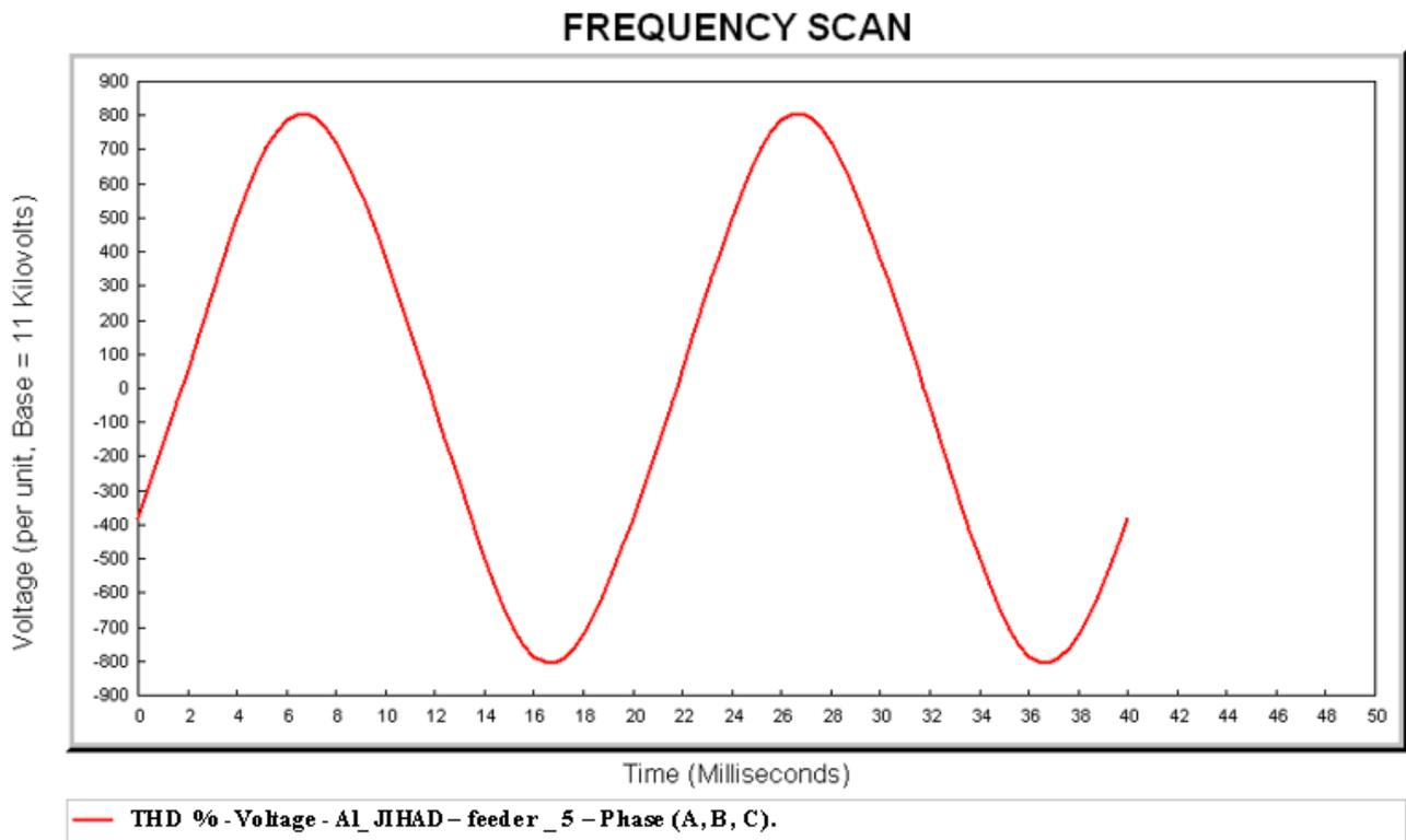
Figure 12. The wave form of voltage before Compensation
