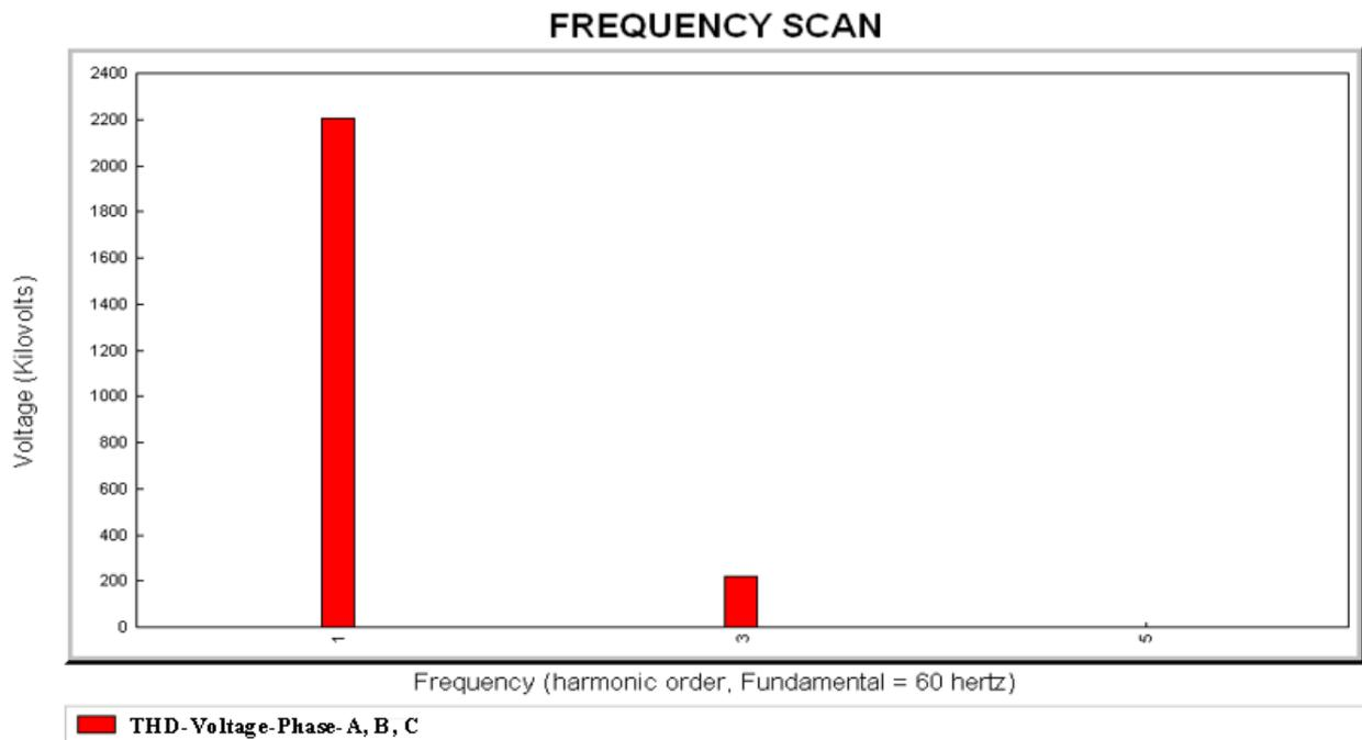
Figure 5. Harmonic order of voltage before Compensation.
