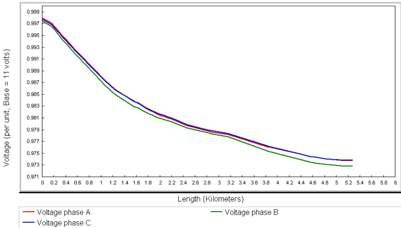
Figure 17. Voltage profile for AI\_JIHAD - feeder\_5 after adding capacitor placement.
