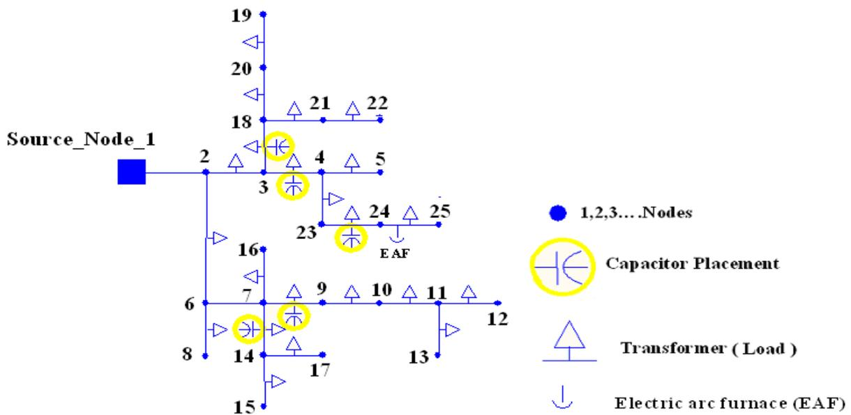
Figure 3. Single Line Diagram of 25 Bus Un-balanced Radial Distribution Network after adding capacitor placement with electric arc furnace (EAF).
