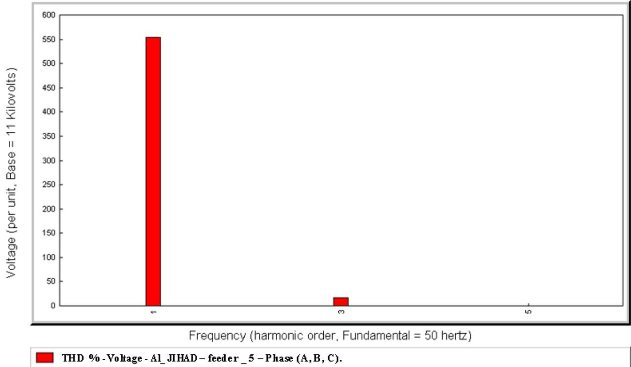
Figure 13. Harmonic order of voltage before Compensation.
