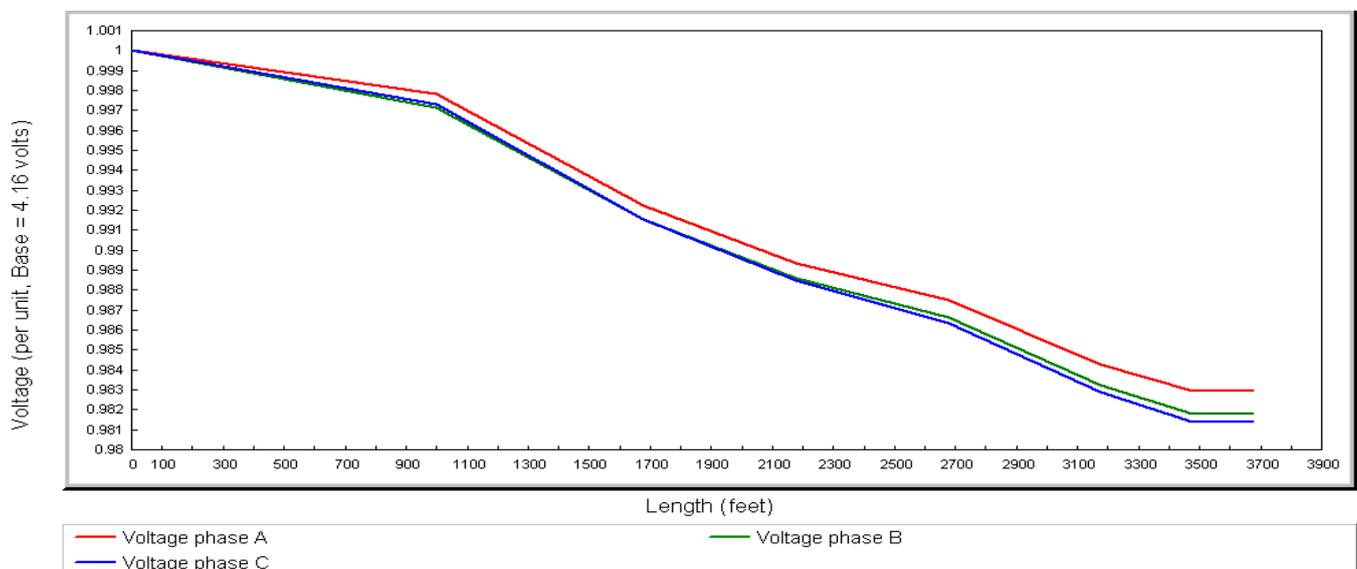
Figure 9. Voltage profile for the 25-Bus Test System un-balanced radial distribution network after Compensation.
