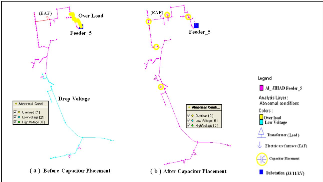
Figure 11. The Abnormal and normal conditions before and after optimal capacitor allocations for Feeder\_5 in AI\_JIHAD distribution network.
