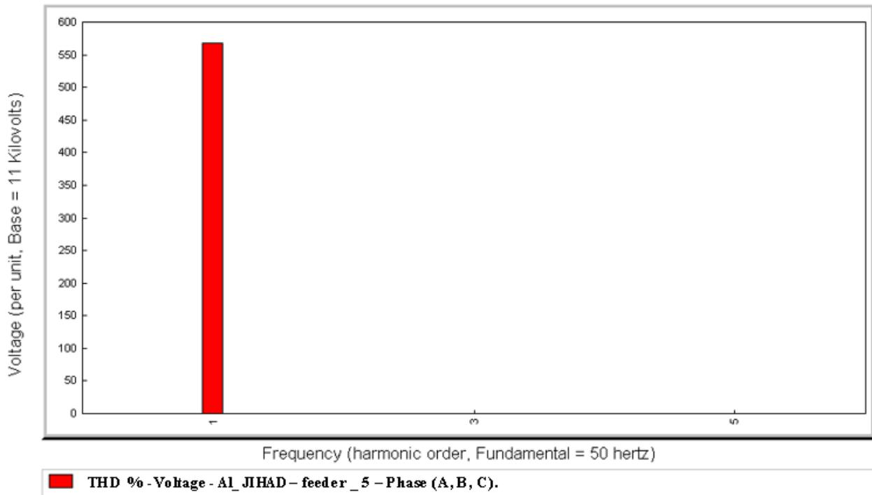
Figure 15. Harmonic order of voltage after Compensation.
