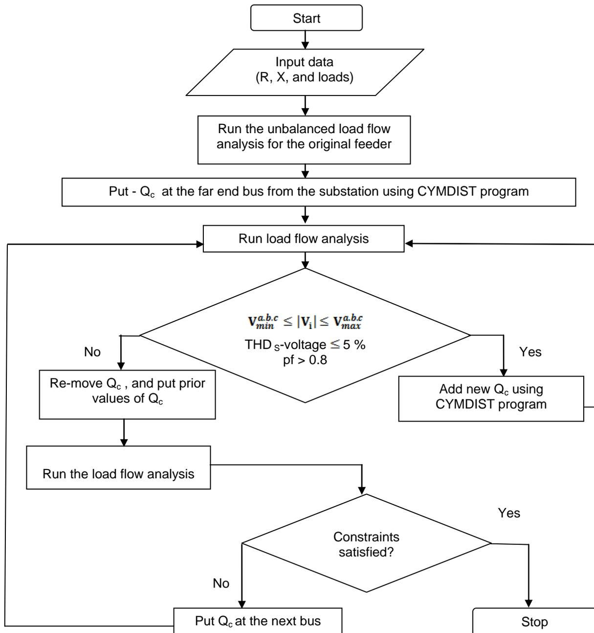
Figure 1. Flowchart of capacitor placement for the search of best suitable location and sizing in un-balanced radial distribution feeder using CYMDIST program.
