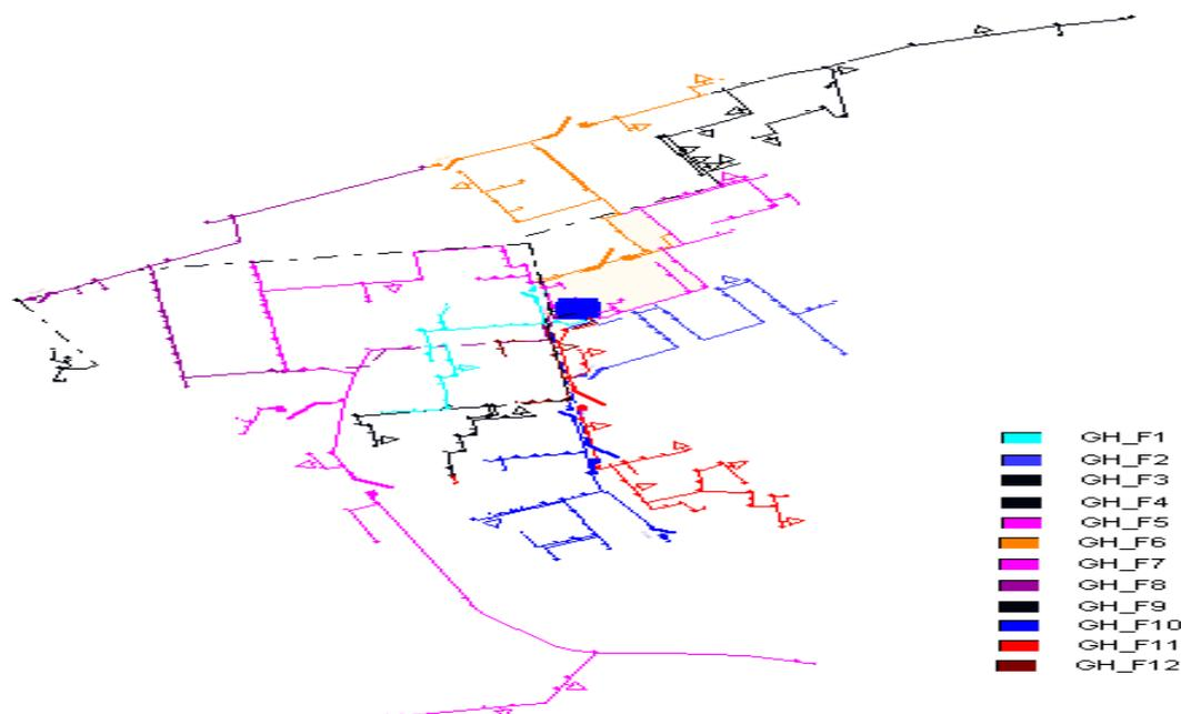
Figure 10. Initial configuration of Al\_ JIHAD distribution network with the secondary transformers (11/0.4 kV).
