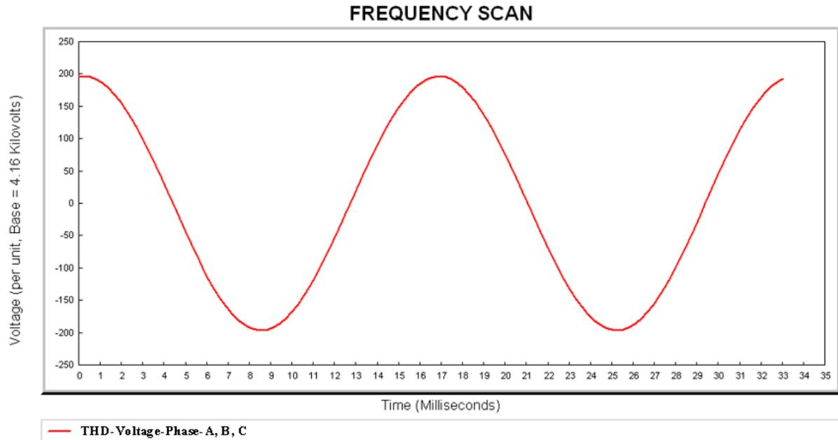
Figure 6. The wave form of voltage after Compensation.
