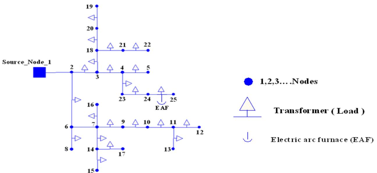
Figure 2. Single Line Diagram of 25 Bus Un-balanced Radial Distribution Network with electric arc furnace (EAF) [11]
