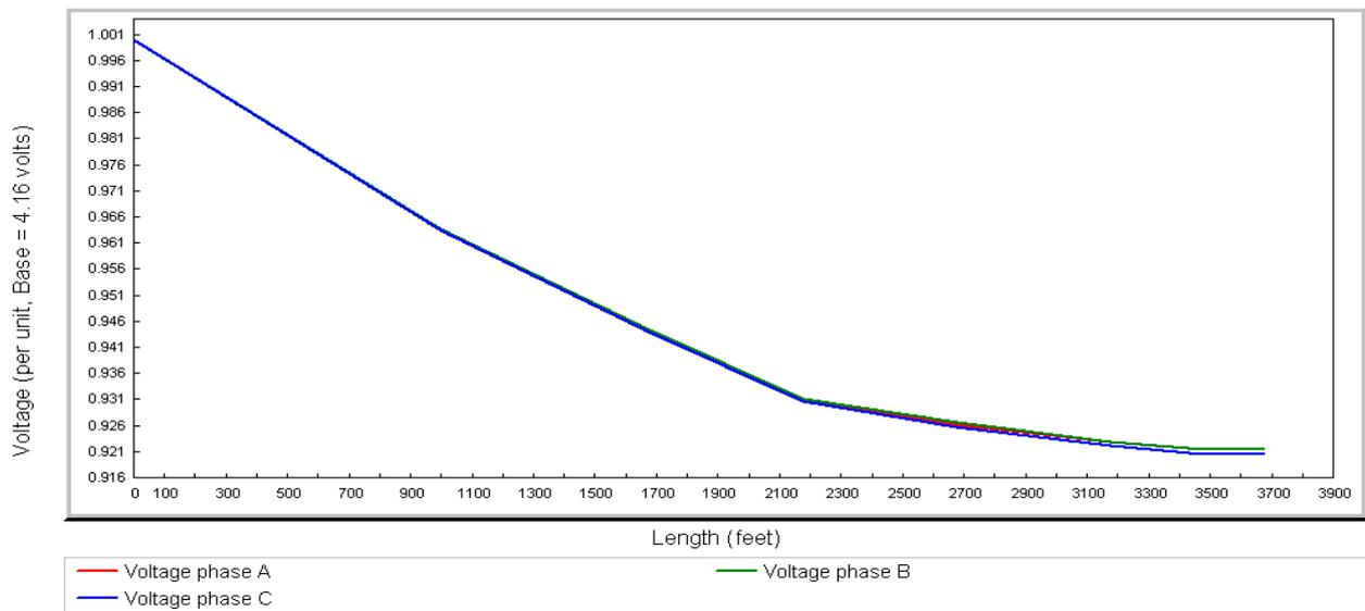
Figure 8. Voltage profile for the 25-Bus Test System un-balanced radial distribution network before Compensation.
