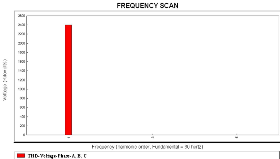
Figure 7. Harmonic order of voltage after Compensation.
