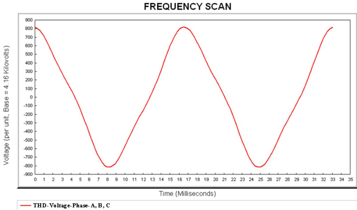
Figure 4. The wave form of voltage before Compensation.
