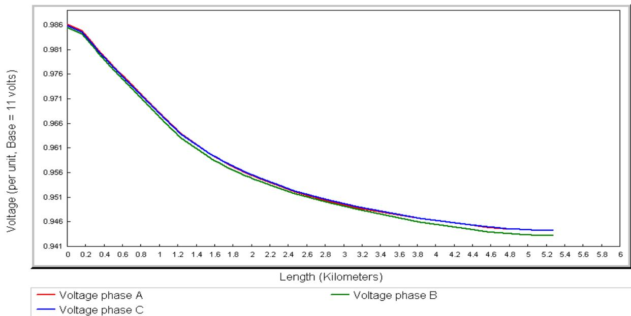
Figure 16. Voltage profile for Al\_ JIHAD - feeder\_5 before adding capacitor placement.
