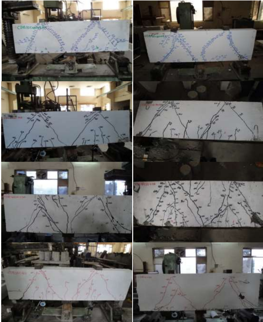
Figure 10: Cracking Patterns of the Tested Beams
