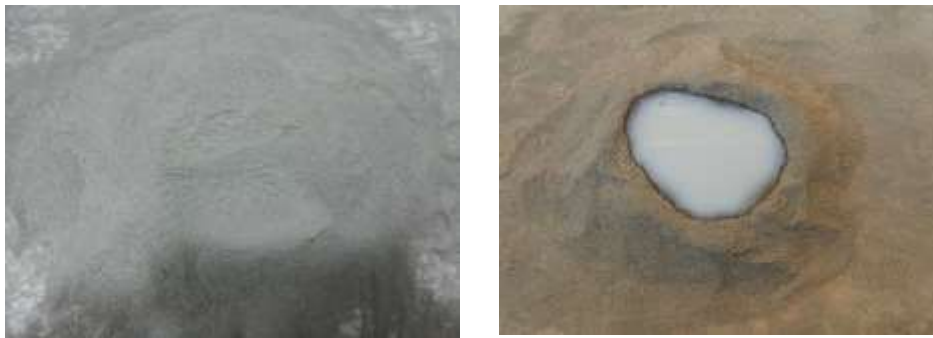
Figure (1): The mixture of cement mortar (a) dry state (b) with nano-materials addition.
