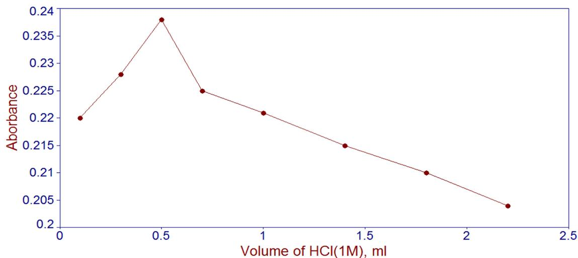
Figure 3A: Effect of various volumes of 1M of HCl on the absorbance of colored product.
