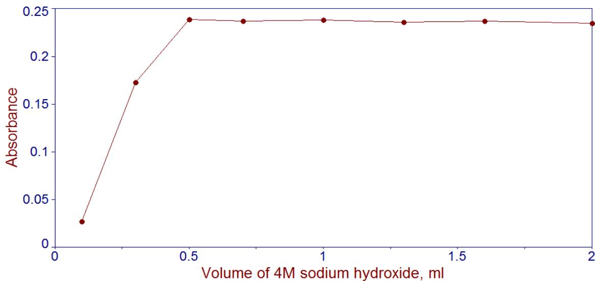
Figur 3D: Effect of volumes of 4M NaOH on the absorbance of azo dye product.
