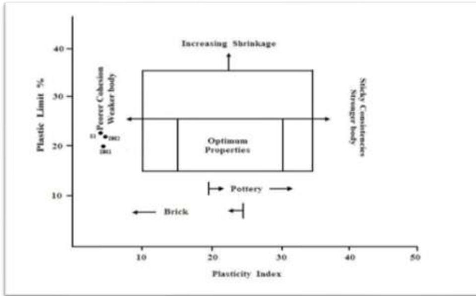
**Figure 3-** Distribution of the studied sites on the plan of the validity of mud according to the British Geological Survey of the [13].
